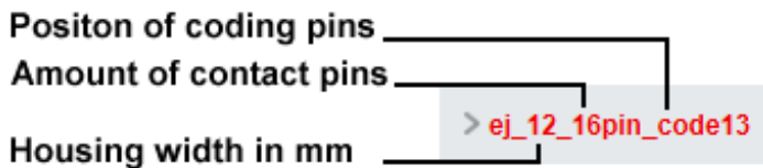
Fig. 25: Naming of the technical drawings
