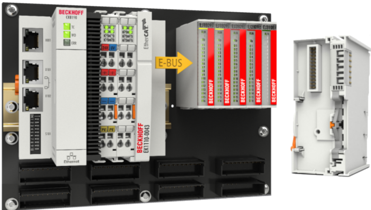
Fig. 22: Example PCB with Embedded PC, EK1110-0043 and EJxxxx, rear view EK1110-0043
