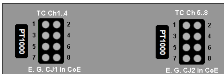
Fig. 13: Routing of the TCs to two different TC connectors using the example of EJ3318
