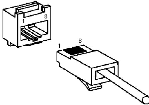
**Figure 14: RJ45 Connector**
