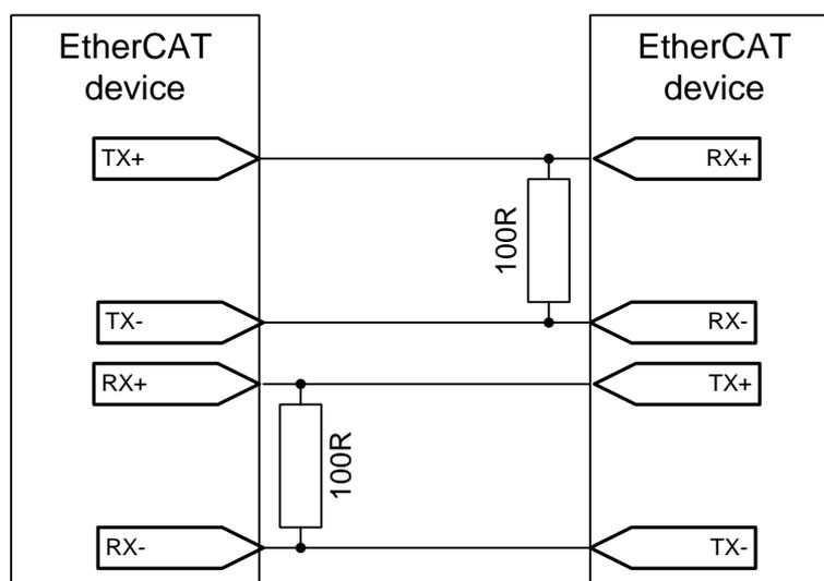
Figure 21: EBUS Connection
