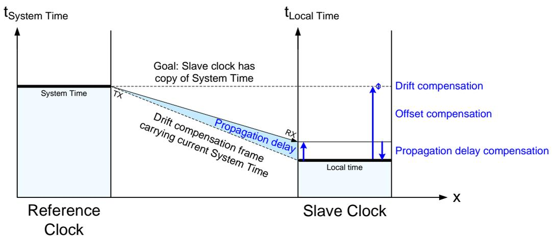
Figure 29: Propagation Delay, Offset, and Drift Compensation
