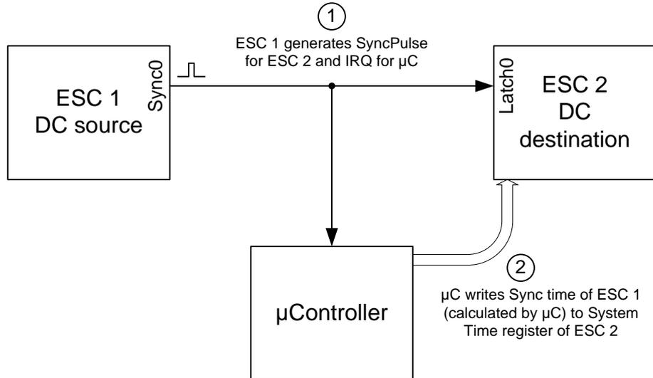
Figure 35: System Time PDI Controlled with two steps
