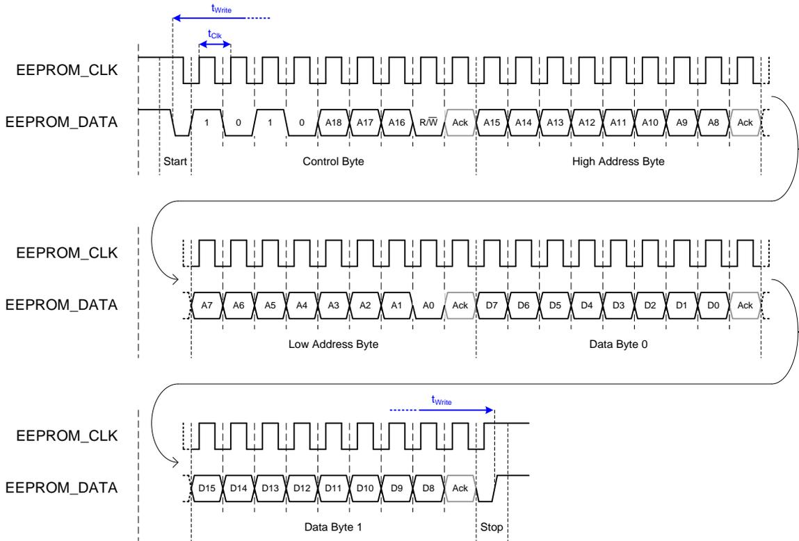
**Figure 41: Write access (2 address bytes, 32 Kbit - 4 Mbit EEPROMs)**
