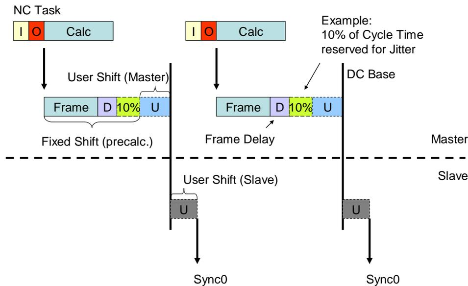
Figure 36: DC Timing Signals in relation to Communication
