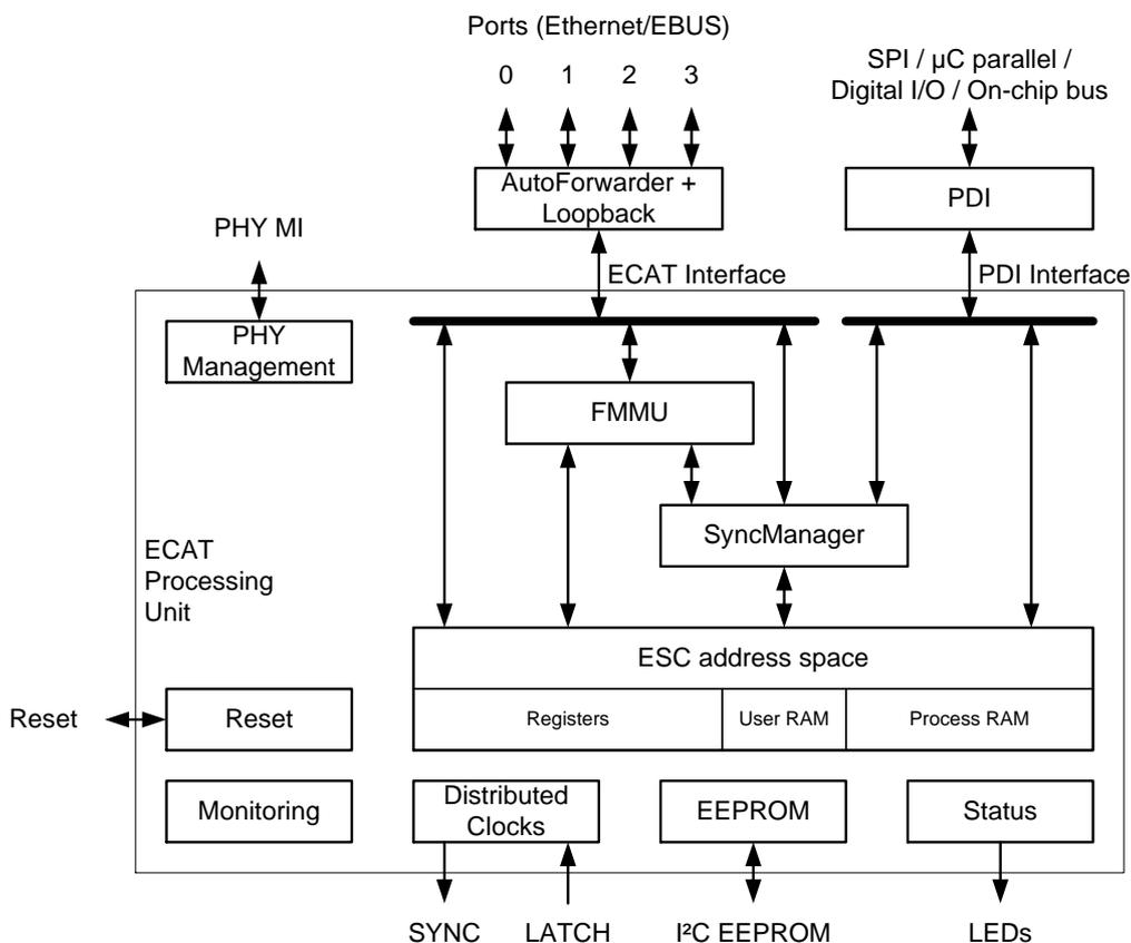
Figure 1: EtherCAT Slave Controller Block Diagram
