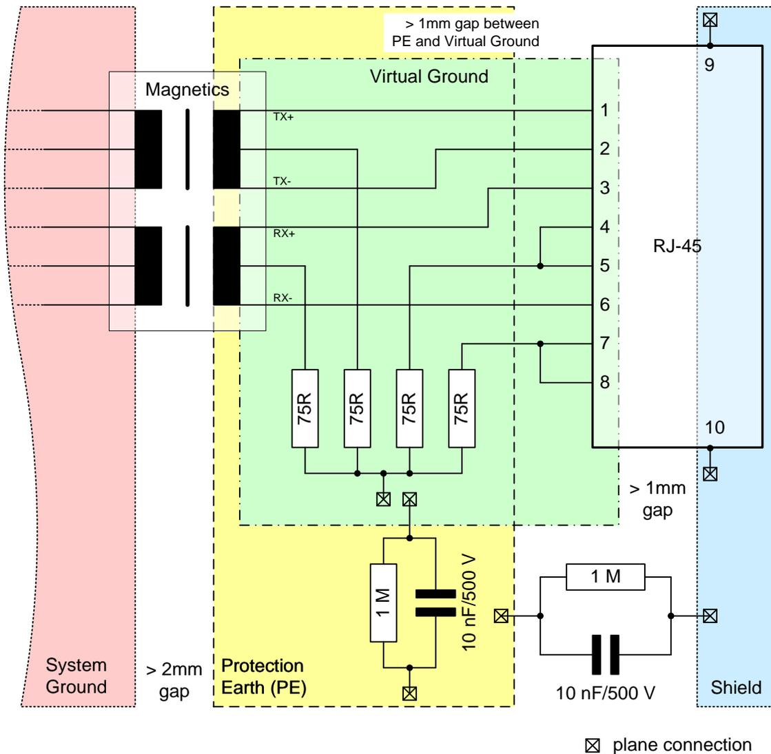
Figure 16: Termination and Grounding Recommendation
