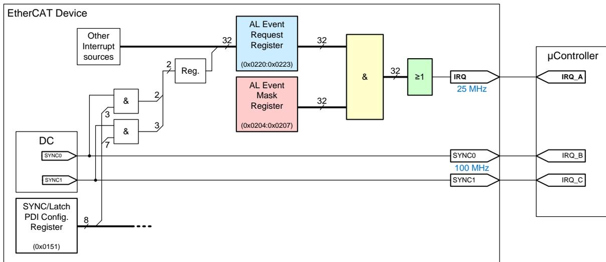
Figure 43: PDI Interrupt Masking and interrupt signals
