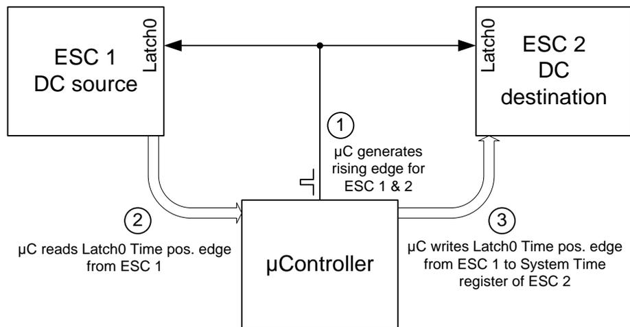
Figure 34: System Time PDI Controlled with three steps
