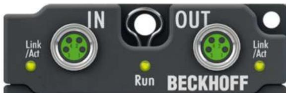
Abb. 8: EtherCAT - Status-LEDs
