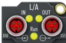
Fig. 4: Status LEDs for EtherCAT
