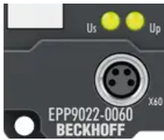
Fig. 3: Status LEDs for the supply voltages
