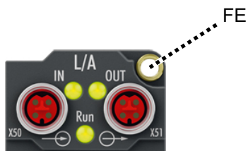
Fig. 1: Connection for functional earth (FE)
