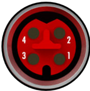
Fig. 7: Pin assignment M8, EtherCAT P In and EtherCAT P Out
