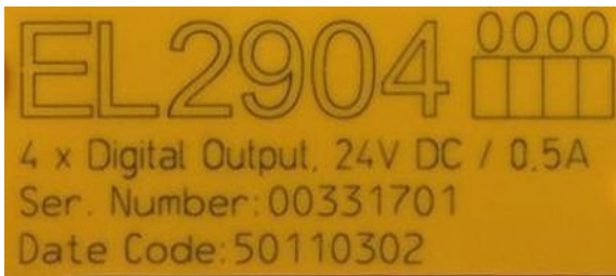
Fig. 20: EL2904 IP20 safety terminal with batch number/ date code 50110302 and unique serial number 00331701
