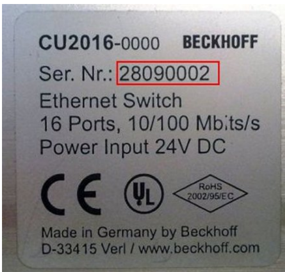
Fig. 16: CU2016 switch with serial/ batch number
