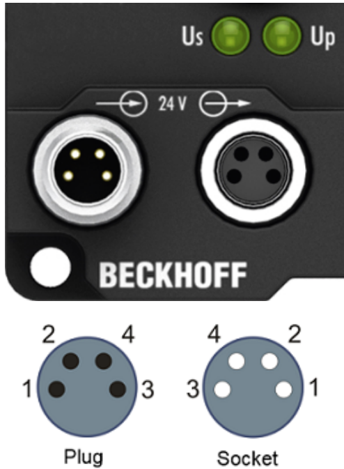
Fig. 10: Connections for the supply voltages
