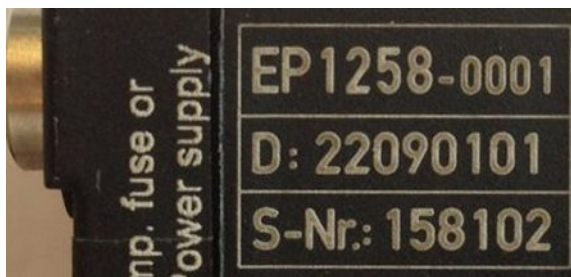
Fig. 14: EP1258-00001 IP67 EtherCAT Box with batch number/ date code 22090101 and unique serial number 158102
