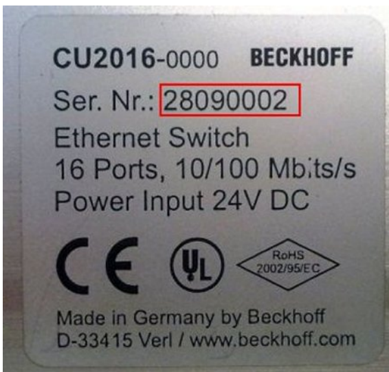
Fig. 12: CU2016 switch with serial/ batch number
