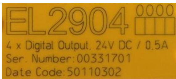
Fig. 16: EL2904 IP20 safety terminal with batch number/ date code 50110302 and unique serial number 00331701
