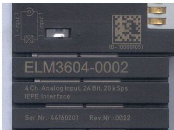
Fig. 17: ELM3604-0002 terminal with unique ID number (QR code) 100001051 and serial/ batch number 44160201
