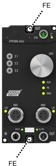
Fig. 4: Functional earth via the fastening holes
