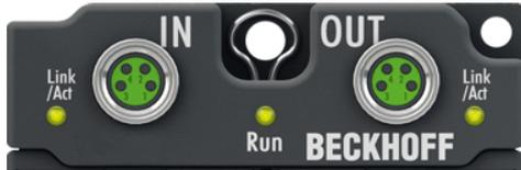
Abb. 6: EtherCAT Status-LEDs
