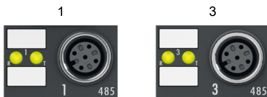
Abb. 8: RS422 / RS485 Status-LEDs
