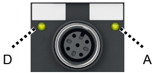
Fig. 11: Status LEDs for signal inputs and outputs
