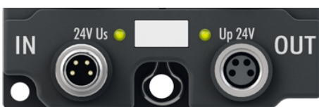
Fig. 10: Status LEDs for the supply voltages
