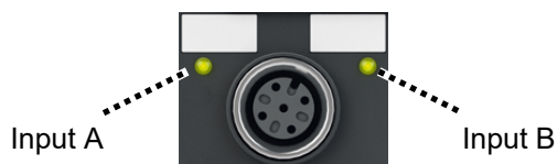
Fig. 10: Status LEDs at M12 sockets
