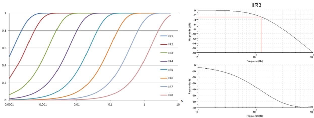
Fig. 5: Step response and Bode diagram of the IIR filter
