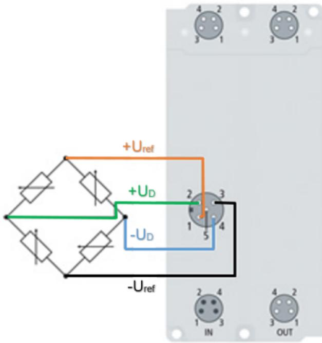
Fig. 22: EP3356: Connection of the load sensor/full bridge
