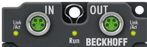
Fig. 10: EtherCAT connectors
