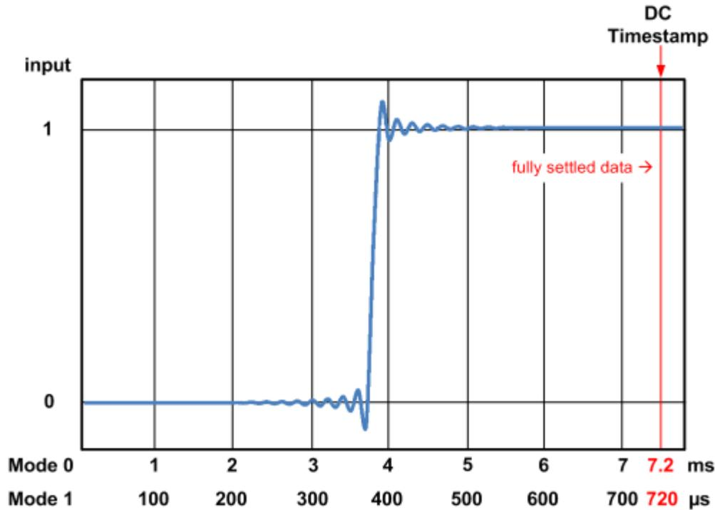
Fig. 7: Latency of the Analog-to-Digital converter
