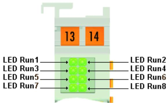
Abb. 7: KL3448 - Diagnose-LEDs
