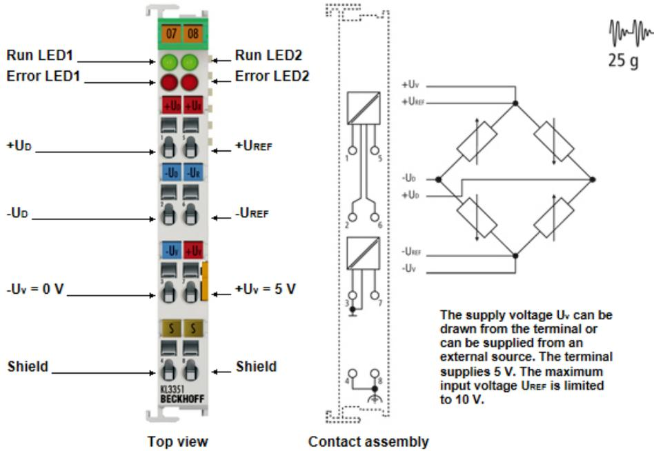
Fig. 10: KL3351 - Contact assignment and LED description
