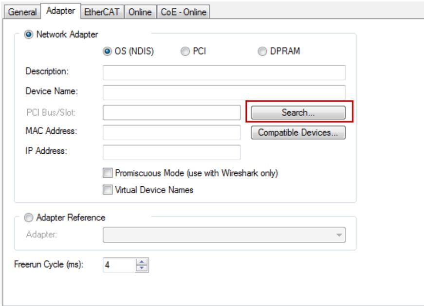
Fig. 14: Search of the existing HW configuration for the EtherCAT configuration of the example
