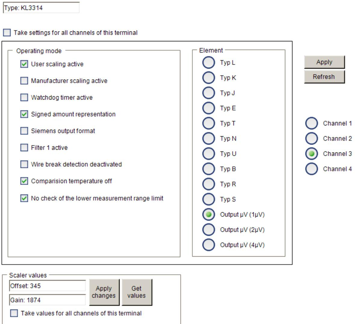
Fig. 12: Settings of KL3314 via visualization of TwinCAT 3
