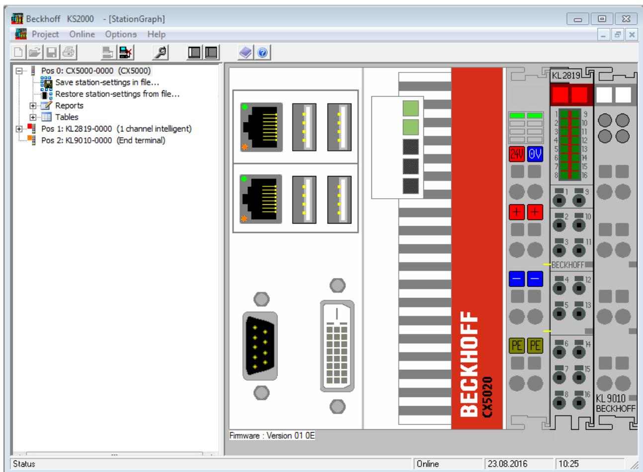
Fig. 19: Display of the fieldbus station in KS2000
