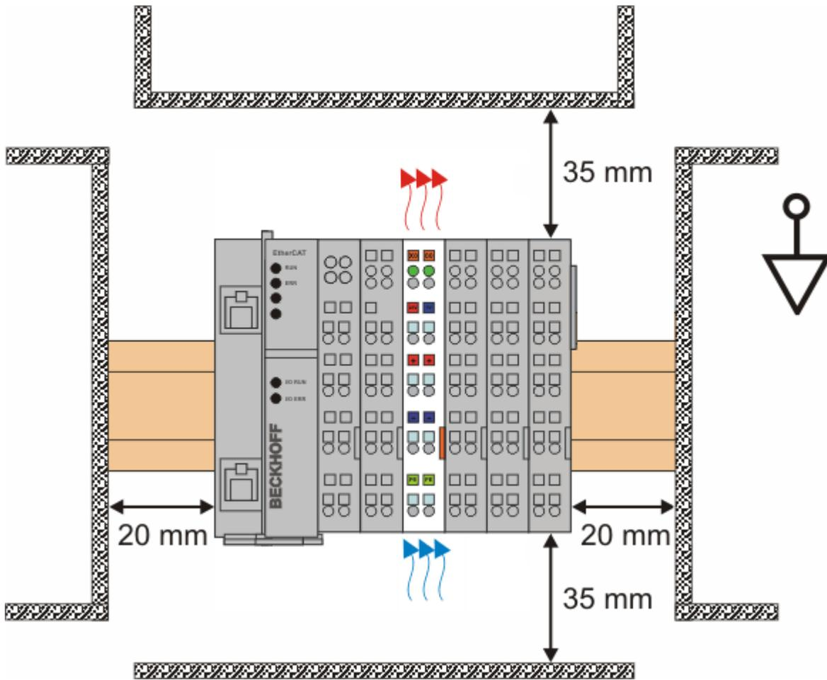
Fig. 16: Recommended distances for standard installation position
