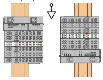
Fig. 15: Other installation positions, example 1
