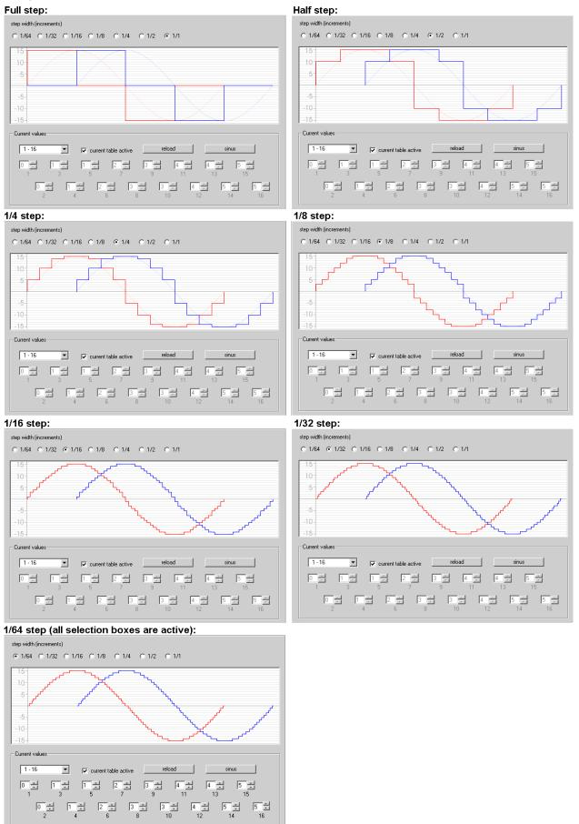
Fig. 35: KL2541 - Examples for current table settings with KS2000
