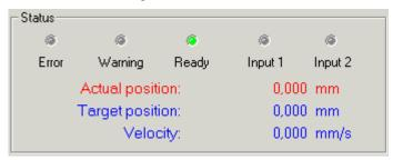
Fig. 40: Status and position display in the Commissioning tab
