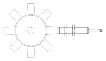
Fig. 5: Pinion with inductive proximity limit switch (register R51 = 8)
