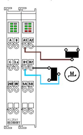
Fig. 26: KL2541 - Bipolar control of an unipolar motor
