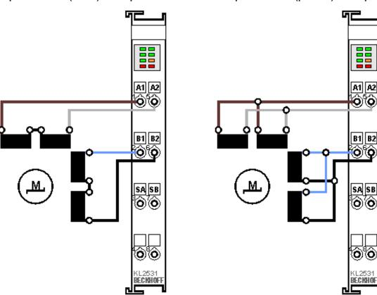
Fig. 22: KL2531 - Bipolar serial (left) and parallel (right) control of a bipolar motor
