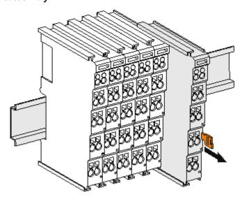
Fig. 11: Disassembling of terminal
