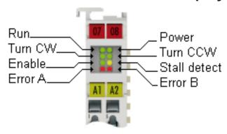
Fig. 2: KL2531 LEDs
