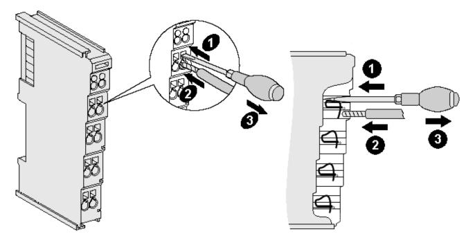
Fig. 20: Connecting a cable on a terminal point
