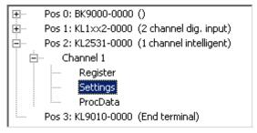
Fig. 30: KS2000 tree branches for channel 1 of the KL2531
