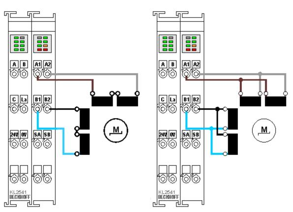
Fig. 25: KL2541 - Bipolar serial (left) and parallel (right) control of a bipolar motor
