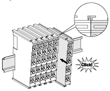
Fig. 10: Attaching on mounting rail
