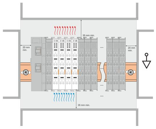
Fig. 13: Recommended distances of installation position for operating without fan
