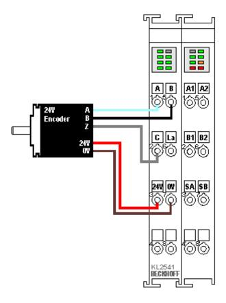
Fig. 27: KL2541 - Connecting an encoder
