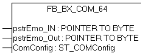
Fig. 123: Function block FB_BX_COM_64
