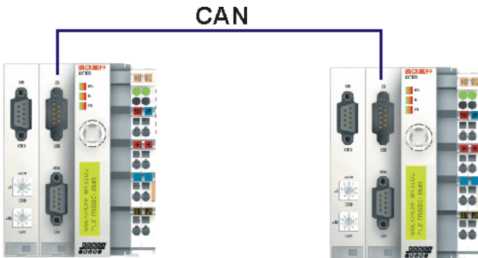
Fig. 77: Communication between BX controllers (via SSB)
