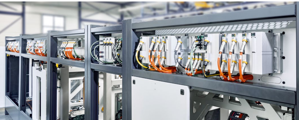
The back of the system is particularly interesting for automation engineers, as each machine module has its own MX-System baseplate onto which the various function modules are attached and screwed.
