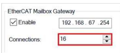
Fig. 4: EtherCAT Mailbox Gateway Connections
