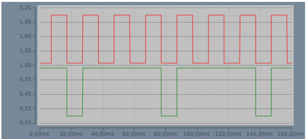
Fig. 30: Example of the signal curve of the input signal in the operating mode Two Channel Async Velocity Control
