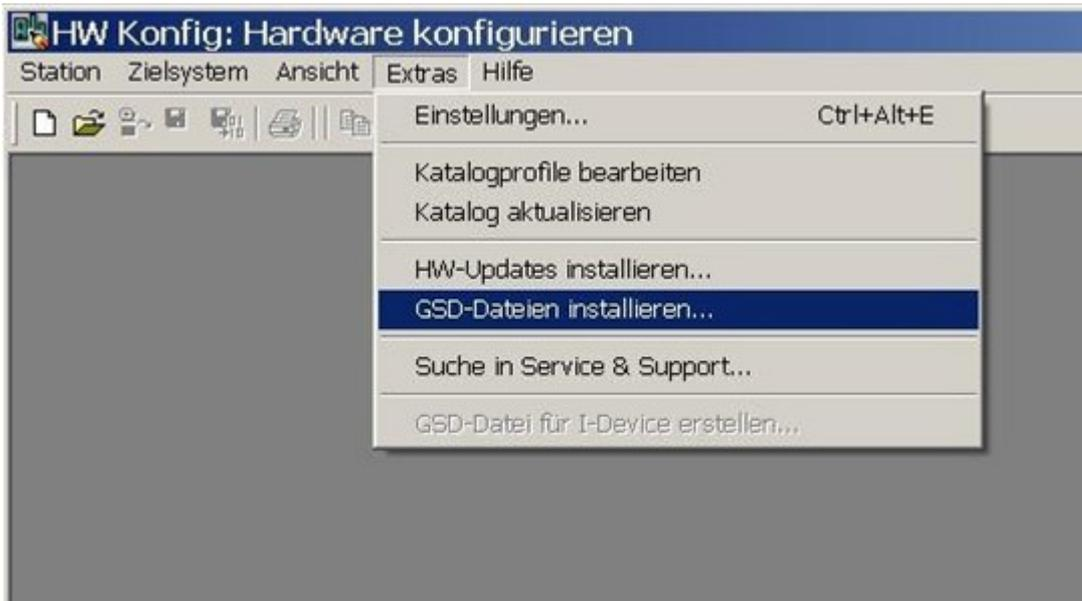
Fig. 48: Installing the EL6930 in Step7
