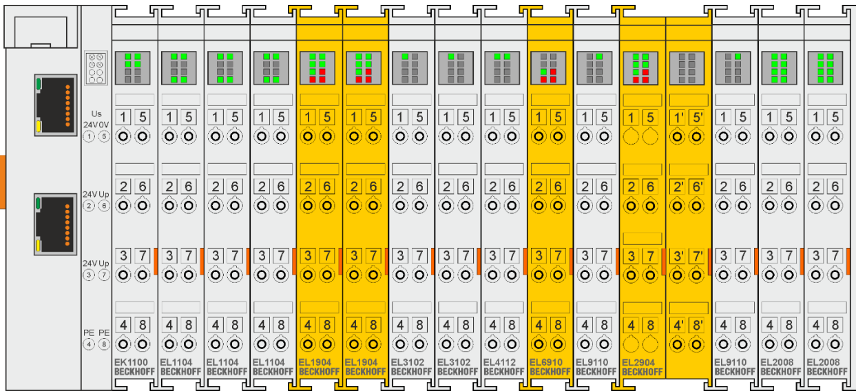
Fig. 4: Sample configuration for temperature measurement
