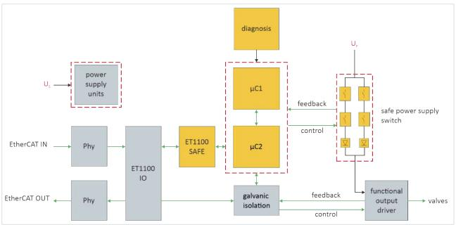
The TwinSAFE component has an internal two-channel structure based on a 1002 structure.
