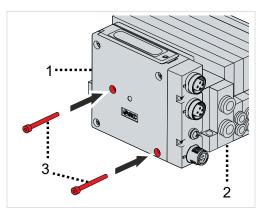
3. Turn the screws [3] into the holes in the head station [1] to screw the head station [1] and the valves [2] together
