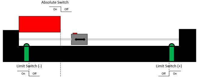
The "..Detection" version of this function block does not manipulate the current position of the axis at the end of the sequence, but instead returns the detected position to the user as "RecordedPosition".
