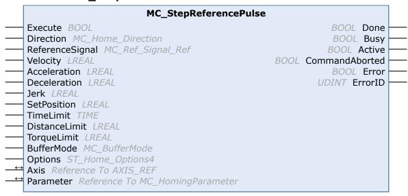
This function block performs the search for a zero pulse of an encoder.
