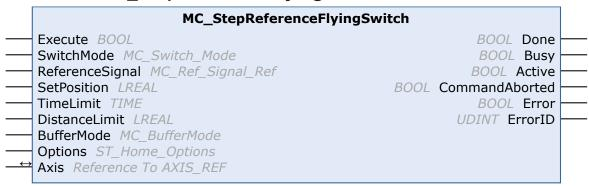
The function block MC\_StepReferenceFlyingSwitch performs referencing during a running movement via an absolutely positioned external physical switch.
