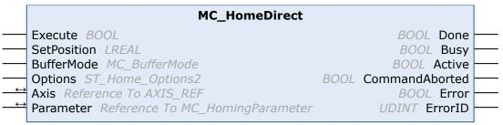
The MC\_HomeDirect function block completes a successful homing sequence, resets the axis to a defined value and ensures that modified parameters are reset to their original values. The axis leaves the homing state.
