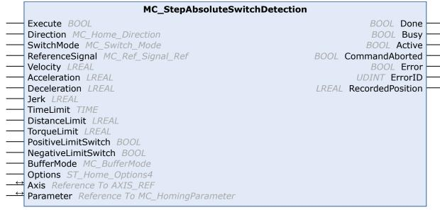
This function block searches for an absolutely positioned, external physical switch.
