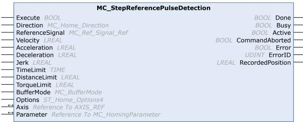
This function block performs the search for a zero pulse of an encoder.
