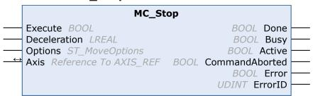
The function block MC\_Stop stops an axis with a defined deceleration ramp and locks the axis against other motion commands. The function block is therefore suitable for stops in special situations, in which further axis movements are to be prevented.
