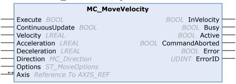
The function block MC\_MoveVelocity starts an endless travel with a specified velocity and direction. The movement can be stopped through a Stop command.
