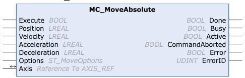
The function block MC\_MoveAbsolute starts the positioning to an absolute target position and monitors the axis movement over the entire travel path. The "Done" output is set once the target position has been reached. Otherwise, the output "CommandAborted" or, in case of an error, the output "Error" is set.
