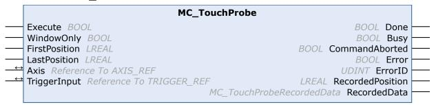
The function block MC\_TouchProbe records an axis position at the time of a digital signal (touch probe function). The position is captured via an external hardware latch and is therefore highly accurate and independent of the cycle time. The function block controls this mechanism and determines the externally recorded position.
