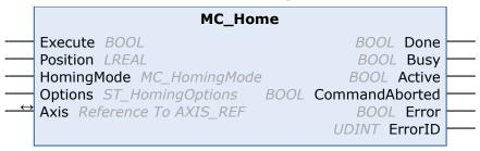
An axis reference run is carried out with the function block MC\_Home.
