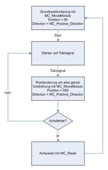
Alternatively, the reset step may be carried out at the start of the step sequence, so that the axis is initialized at the start of the process.
