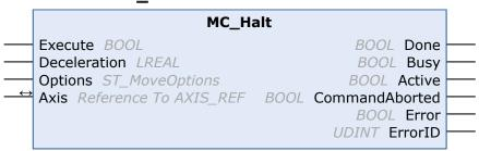
The function block MC\_Halt stops an axis with a defined deceleration ramp.
