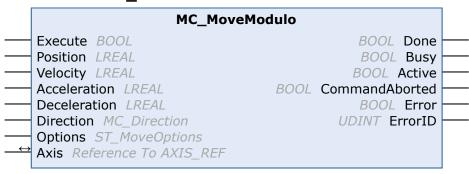
The function block MC\_MoveModulo is used to execute a positioning operation, which refers to the modulo position of an axis. The basis for a modulo rotation is the adjustable parameter "Modulo Factor" of the AXIS\_REF structure (Axis.Parameter.ModuloFactor, e.g. 360°). A distinction is made between three possible start types, depending on the "Direction" input.
