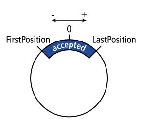
examples of windows, where trigger events are accepted (for modulo axes)
