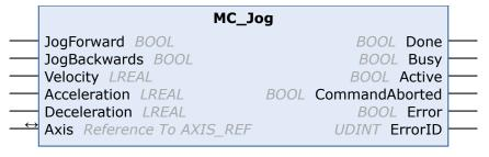
The function block MC\_Jog enables an axis to be moved via manual keys. The key signal can be linked directly with the "JogForward" and "JogBackwards" inputs.
