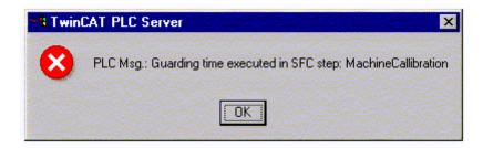
With this, the PLC programmer inserts the string stored in the variable strSFCErrorStep into the message. The insertion point is marked by the %s characters in the format string.
