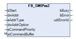
The function block FB\_SMIPos2 controls the movement to the fixed position *Pos2* configured on the motor side. *Pos2* can be read and changed using the function blocks <u>FB\_SMIPos2Read()</u> [ $\blacktriangleright$ \_30] and <u>FB\_SMIPos2Write()</u> [ $\blacktriangleright$ \_31].
