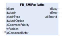
The function block FB\_SMIPos1Write writes the fixed position *Pos1* that can be configured on the motor side. *Pos1* can be read with the function block <u>FB\_SMIPos1Read()</u> [ $\blacktriangleright$ \_26].
