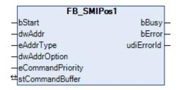
The function block FB\_SMIPos1 realizes the movement to the fixed position *Pos1* configured on the motor side. *Pos1* can be read and changed using the function blocks <u>FB\_SMIPos1Read()</u> [ $\blacktriangleright$ \_26] and <u>FB\_SMIPos1Write()</u> [ $\blacktriangleright$ \_27].
