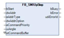
The function block FB\_SMIUpStep controls the motor run upwards by a specified angle (0-510 degrees).
