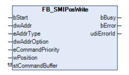
The function block FB\_SMIPosWrite moves the drive to the specified position.
