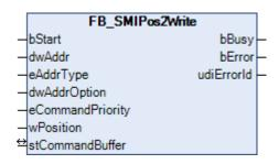
The function block FB\_SMIPos2Write writes the fixed position *Pos2* that can be configured on the motor side. *Pos2* can be read with the function block <u>FB\_SMIPos2Read()</u> [ $\blacktriangleright$ \_30].
