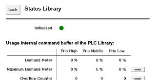
Communication between the individual PLC blocks and the Bus Terminal takes place within the PLC library via three central buffers (for each SMI terminal). The extent of utilisation of the buffers and possible overflows can be determined from the illustrated table.
