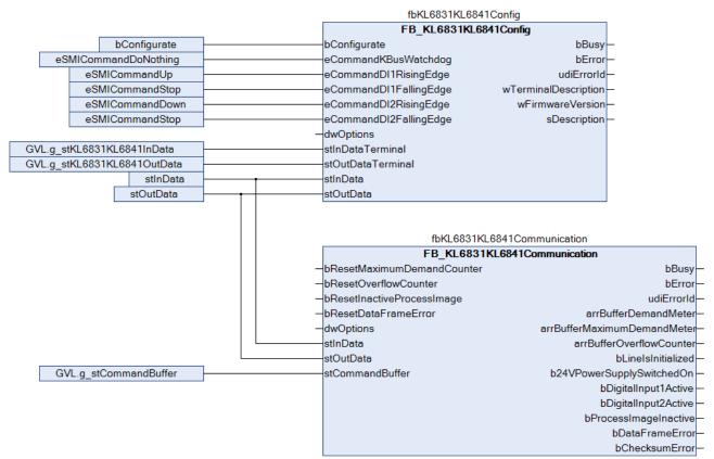
The function block FB\_KL6831KL6841Config() is linked to the process image of the KL6831/KL6841. Once the configuration is complete, the function block FB\_KL6831KL6841Communication() receives the process values of the KL6831/KL6841. No SMI commands can be sent while the configuration is in progress.
