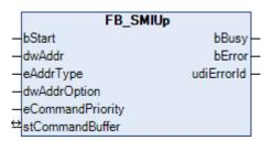
The function block FB\_SMIUp controls the motor run up to the upper end position.
