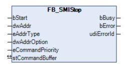
The function block FB\_SMIStop stops the motor run.
