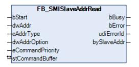
The function block FB\_SMISlaveAddrRead reads the address (0-15) of a drive.
