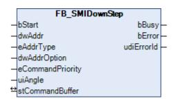
The function block FB\_SMIDownStep controls the motor run downwards by a specified angle (0-510 degrees).
