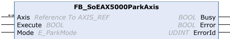
This function block enables the parking functionality of an AX5000. A parked channel of an AX5000 is temporarily disabled.
