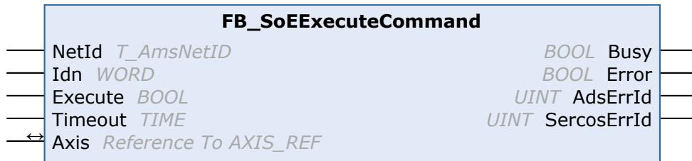
With the FB\_SoEExecuteCommand function block a command can be executed.
