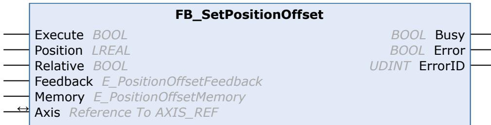
The FB\_SetPositionOffset function block can be used to store a position offset in the memory of a Beckhoff servo hardware. Saving in the digital nameplate of the connected motor encoder is also possible. To do this, the offset must first be configured with the [DriveManager](#) and then the same memory location (encoder / drive) must be used in the function block.
