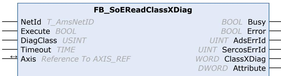
With the function block FB\_SoEReadClassXDiag, the current Class 1 diagnosis (S-0-0011) ... Class 3 diagnosis (S-0-0013) can be read out as WORD. There is the conversion function F\_ConvWordToSTAX5000C1D for the evaluation of the Class 1 diagnosis as a structure ST\_AX5000\_C1D, (see TwinCAT 3 PLC Lib Tc2\_Drive documentation).
