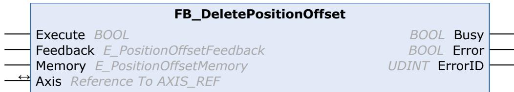
The FB\_DeletePositionOffset function block can be used to delete a position offset in the memory of a Beckhoff servo hardware.
