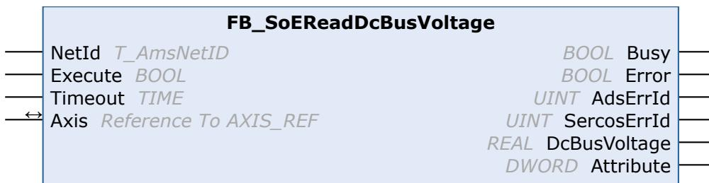
With the FB\_SoEReadDcBusVoltage function block the Dc-Bus voltage of the drive (S-0-0380) can be read.
