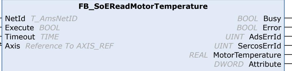
With the function block FB\_SoEReadMotorTemperature the temperature of the motor (S-0-0383) can be read. If the motor does not contain a temperature sensor, this is 0.0, i.e. 0.0 °C.
