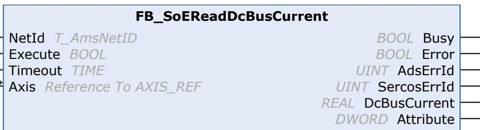
With the FB\_SoEAX5000ReadDcBusCurrent function block the DC-Bus current (S-0-0381) can be read.
