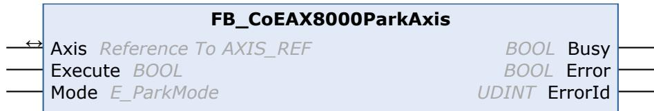
This function block enables the parking functionality of an AX8000. A parked channel of an AX8000 is temporarily disabled.
