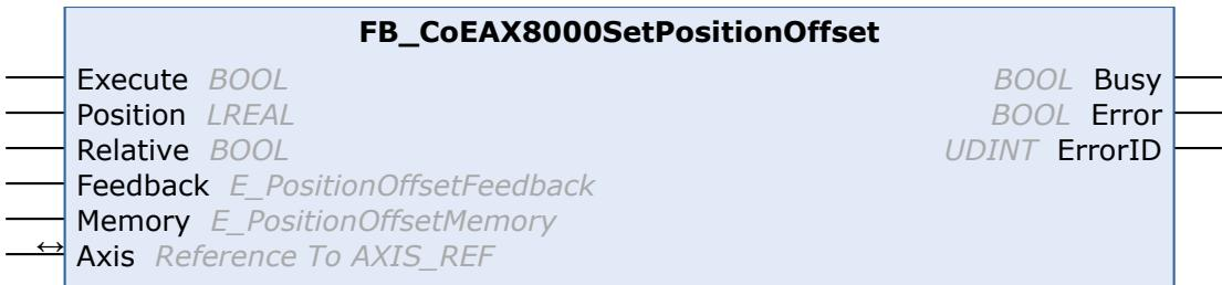
With the FB\_CoEAX8000SetPositionOffset function block, a position offset can be saved in the memory of the AX8000 or of the digital nameplate of the connected motor encoder. To do this, the offset must first be configured with the [DriveManager](#) and then the same memory location (encoder / drive) must be used in the function block.
