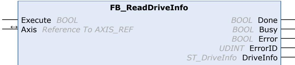
The FB\_ReadDriveInfo function block can be used to read basic information for communication with a Beckhoff servo hardware.
