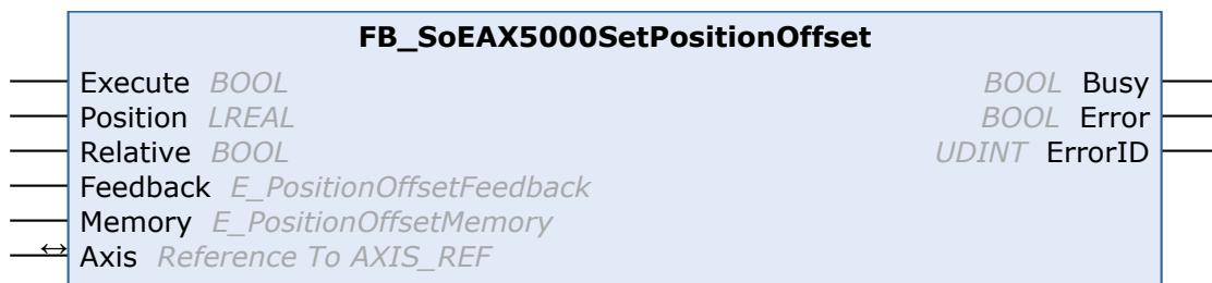
With the function block FB\_SoEAX5000SetPositionOffset a position offset can be saved in the memory of the AX5000 or of the digital nameplate of the connected motor encoder. To do this, the offset must first be configured with the [DriveManager](#) and then the same memory location (encoder / drive) must be used in the function block.
