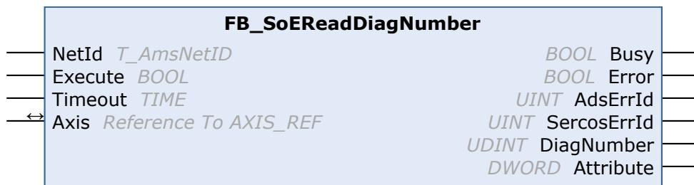
With the FB\_SoEReadDiagNumber function block the current diagnostic number can be read out as UDINT (S-0-0390).
