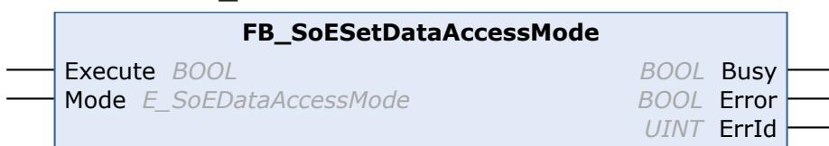
The SoE parameter access mode is set with the function block FB\_SoESetDataAccessMode. Attributes & Value are accessed in parallel by default. If this access mode is not supported by the device manufacturer, sequential access can be enforced. Generally, however, parallel access is faster.
