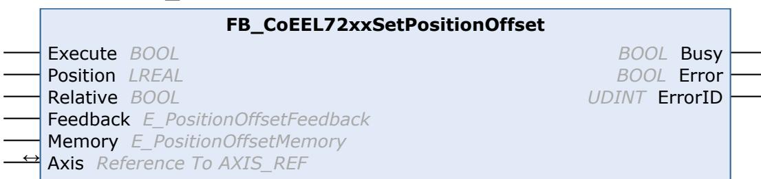
With the function block FB\_CoEEL72xxSetPositionOffset, a position offset can be saved in the memory of the EL72xx. Saving in the digital nameplate of the connected motor encoder is currently not planned.
