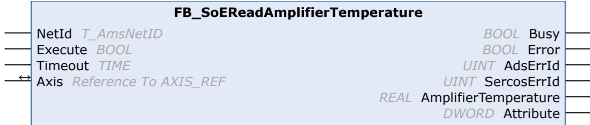
With the FB\_SoEReadAmplifierTemperature function block the temperature of the drive (S-0-0384) can be read.
