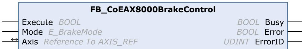
This function block can be used to manually open or close the brake of a motor that is operated on an AX8000.
