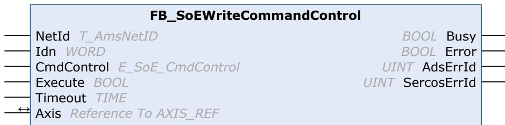
With the FB\_SoEWriteCommandControl function block a command can be prepared, started or canceled.
