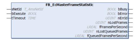
The function block FB\_EcMasterFrameStatistic can be used to read the frame statistics of the EtherCAT master. A distinction is made between cyclic and acyclic (queued) frames. Acyclic frames are used for the initialization or for parameter access to EtherCAT slaves. Frames are regarded as lost if they fail to return to the master or are invalid.
