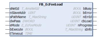
The function block FB\_EcFoeLoad can be used to download or upload files to or from an EtherCAT device via the "File access over EtherCAT" mailbox protocol.
