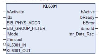
This function block deals with the KL6301 EIB Bus Terminal communication. It is used for configuring the KL6301 and for starting the data exchange with the EIB network.
