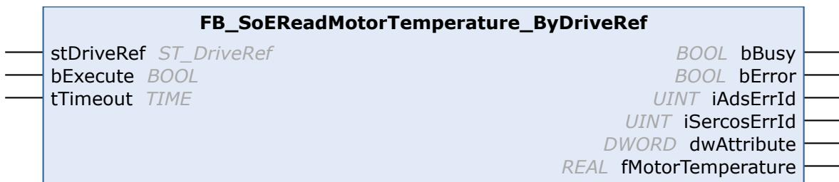
With the function block FB\_SoEReadMotorTemperature\_ByDriveRef the temperature of the motor (S-0-0383) can be read. If the motor does not contain a temperature sensor, this is 0.0, i.e. 0.0 °C.
