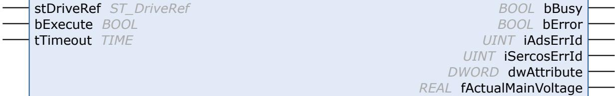
With the FB\_SoEAX5000ReadActMainVoltage\_ByDriveRef function block the current peak value of the mains voltage of the AX5000 (P-0-0200) can be read.
