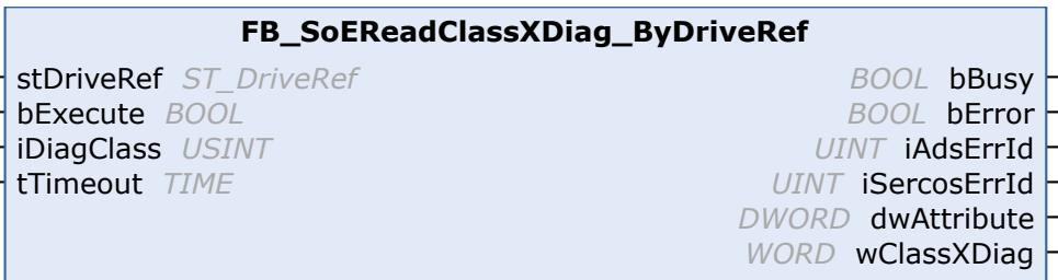
With the FB\_SoEReadClassXDiag\_ByDriveRef function block the current class 1 diagnosis (S-0-0011) ... class 3 diagnosis (S-0-0013) can be read as WORD. For the evaluation of the class 1 diagnosis as structure [ST\\_AX5000\\_C1D](#) [▶ 47] there is a conversion function [F\\_ConvWordToSTAX5000C1D](#) [▶ 30].
