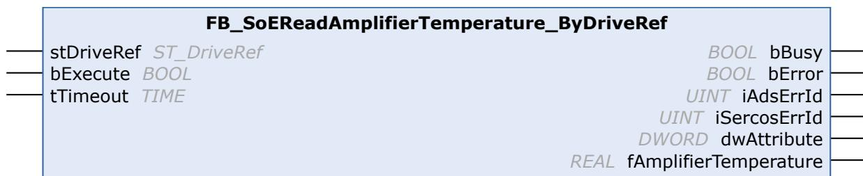
With the FB\_SoEReadAmplifierTemperature\_ByDriveRef function block the temperature of the drive (S-0-0384) can be read.
