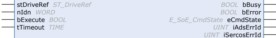
With the FB\_SoEReadCommandState\_ByDriveRef function block the execution of the command can be checked.
