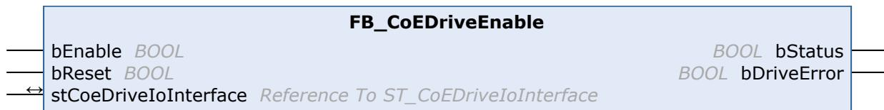
The FB\_CoEDriveEnable function block enables a CoE drive in order to be able to subsequently supply it with setpoints using the function block [FB\\_CoEDriveMoveVelocity](#) [▶ 41].
