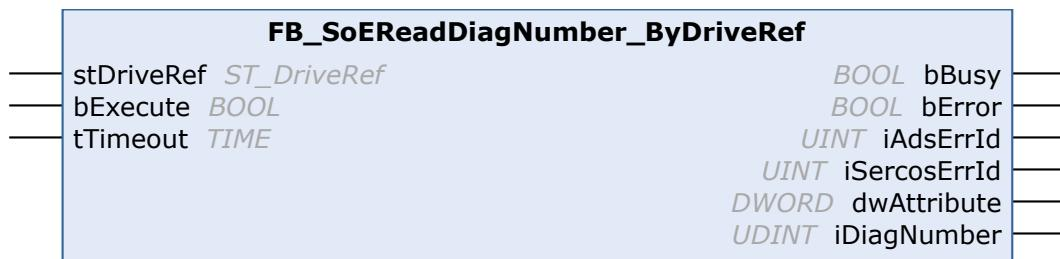
With the FB\_SoEReadDiagNumber\_ByDriveRef function block the current diagnostic number can be read as UDINT (S-0-0390).
