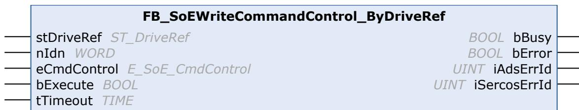
With the FB\_SoEWriteCommandControl\_ByDriveRef function block a command can either be prepared, started or aborted.
