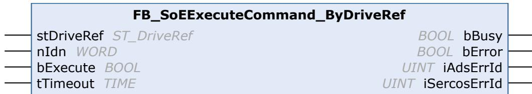
With the FB\_SoEExecuteCommand\_ByDriveRef function block a command can be executed.
