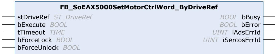
With the FB\_SoEAX5000SetMotorCtrlWord\_ByDriveRef function block the ForceLock bit (Bit 0) and the ForceUnlock bit in the Motor Control Word (P-0-0096) can be set, in order to activate or release the brake. Normally the brake is automatically controlled via the Enable of the drive.
