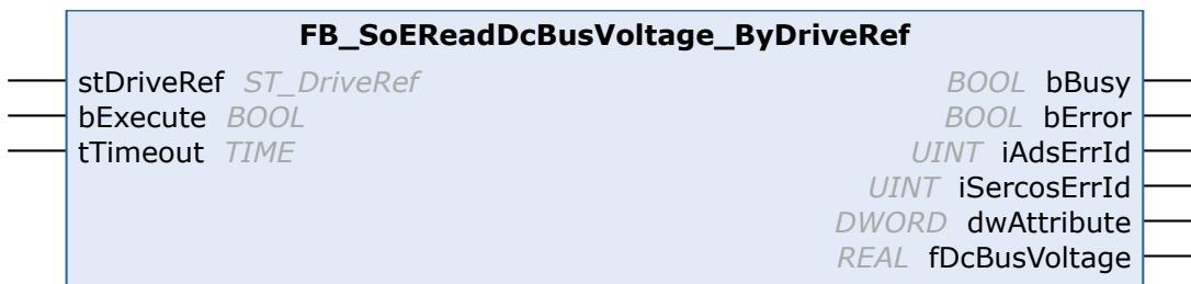
With the FB\_SoEReadDcBusVoltage\_ByDriveRef function block the DC-Bus voltage of the drive (S-0-0380) can be read.
