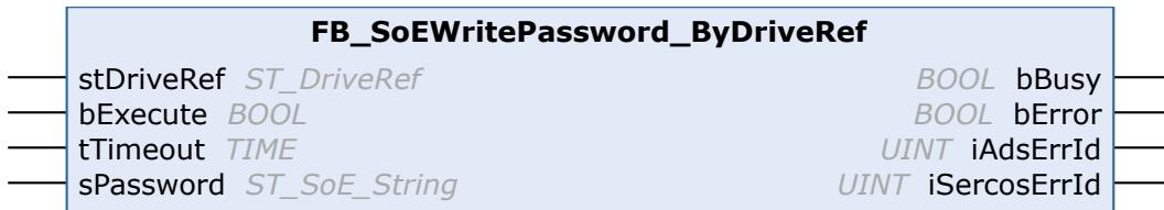
Using the FB\_SoEWritePassword\_ByDriveRef function block the drive password (S-0-0267) can be set.
