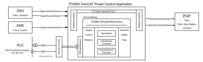
A Beckhoff PGP controller consists of the embedded PC and the grid data acquisition (see <u>Grid data acquisition [17]</u>), as well as the <u>TwinCAT Power Plant Control</u> as the controller kernel in the form of the TwinCAT module <u>TcPowerPlantControl</u>. This module is integrated into a TwinCAT 3 project and provides all the necessary interfaces (see <u>Interfaces [17]</u>) and control functions (see <u>Functions [17]</u>).
