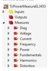
The measurement data is divided into logically separate structures, which can be individually enabled or disabled as required under *Data Area* in the *Enable* column. When starting up, the module automatically recognizes the activated structures and only reads the relevant measured values from the EtherCAT Terminal.
