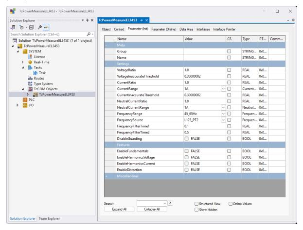
12. This configuration is executed by Activate Configuration and starting TwinCAT on a target system. The bValid under the Measure Data Area in the Diag structure can be used to quickly identify valid measurement data. Otherwise, the messages from TwinCAT should be checked in the Output window.
