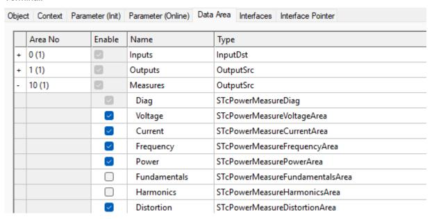
Each of these structures begins with a timestamp (Timestamp), which indicates the time of the last update in distributed clocks time (DC time). This is followed by the diagnostic structure (*Diag*), which contains status information such as when measuring ranges are exceeded or not reached. This is followed by the actual measurement data, which can be divided into further substructures, for example to distinguish between phase-neutral (LN) and phase-phase voltages (LL).
