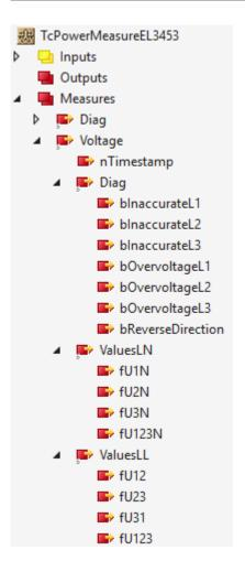
By default, the measured values are output as RMS values per phase and as a total value across all three phases. They are expressed in SI units (e.g. Volt, Ampere, Watt) as floating-point numbers with single precision according to IEEE 754.
