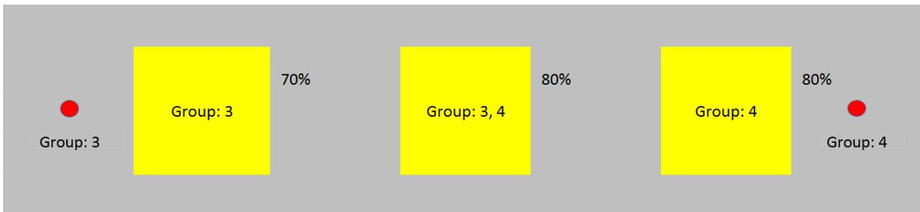
In the following illustration, group 4 no longer has presence. The right-hand lamp is set to the basic value on expiry of the 1<sup>st</sup> overrun time and the middle lamp is reduced to the set value of group 3.
