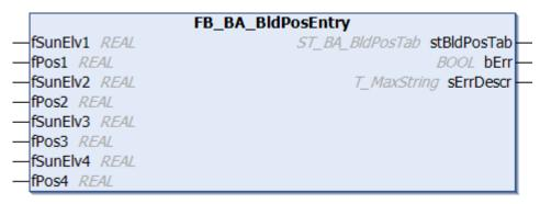
The function block FB\_BA\_BldPosEntry serves for the input of interpolation points for the function block <u>FB\_BARSunProtectionEx [\rightarrow 396]</u>, if this should be operated in the height positioning mode with the help of a table (see E\_BARPosMode).
