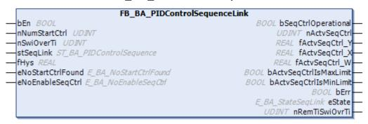
This function block represents the higher-level connection of a sequence control.
