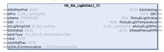
This template is used to control a DALI light actuator, a DALI group or DALI devices with a broadcast, whereby color temperature control is supported.
