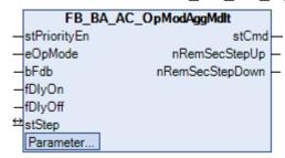
The template serves as a link between the steps within the step sequence control of an air conditioning system.
