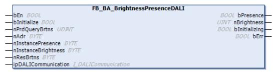
This template is used to read a combined DALI brightness and occupancy sensor.
