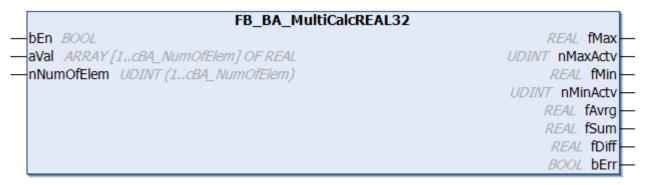
The multi-calculation function block FB\_BA\_MultiCalcREAL32 exists for the variable type REAL.
