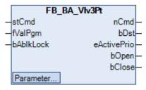
The template is used to control a three-point valve. It mainly consists of the base class <u>FB\_BA\_ActuatorMO\_FB\_991</u>, the function block <u>Anlg3Pnt\_Paths and the anti-blocking protection function Ablk\_9997</u>.
