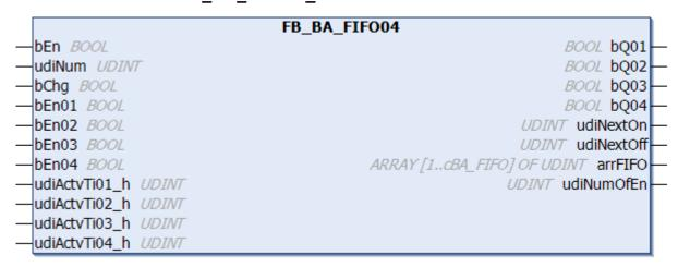
This function block is used to evaluate the FiFo memory from <u>FB\_BA\_FIFO04\_I▶648</u>]. The inputs are linked according to the FIFO table to the corresponding outputs of the function block <u>FB\_BA\_FIFO04\_BOOL</u> or <u>FB\_BA\_FIFO04\_REAL</u>.
