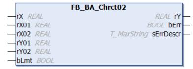
The function block FB\_BA\_Chrct02 represents a linear interpolation with 2 interpolation points and can be used to generate a characteristic curve. The characteristic curve is determined by the interpolation points [rX1/rY1] and [rX2/rY2]. If the input variable bLmt is TRUE, rY is limited by rY01 and rY02. If bLmt is FALSE, rY is not limited.
