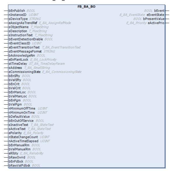
The function block FB\_BA\_BO represents a binary output object within the base framework. The variables for linking the control output to the terminal are available as input or output variables on the function block.
