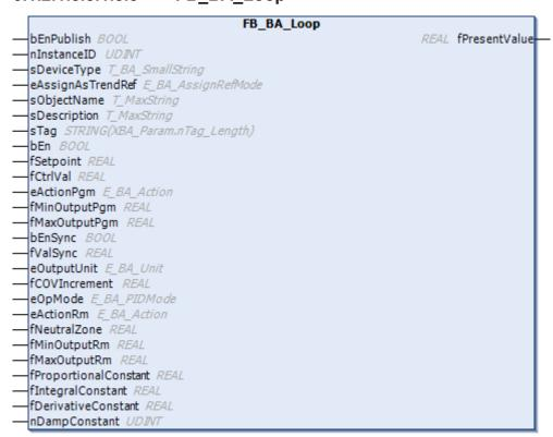
The function block FB\_BA\_Loop represents a PID controller within the project structure of TF8040.
