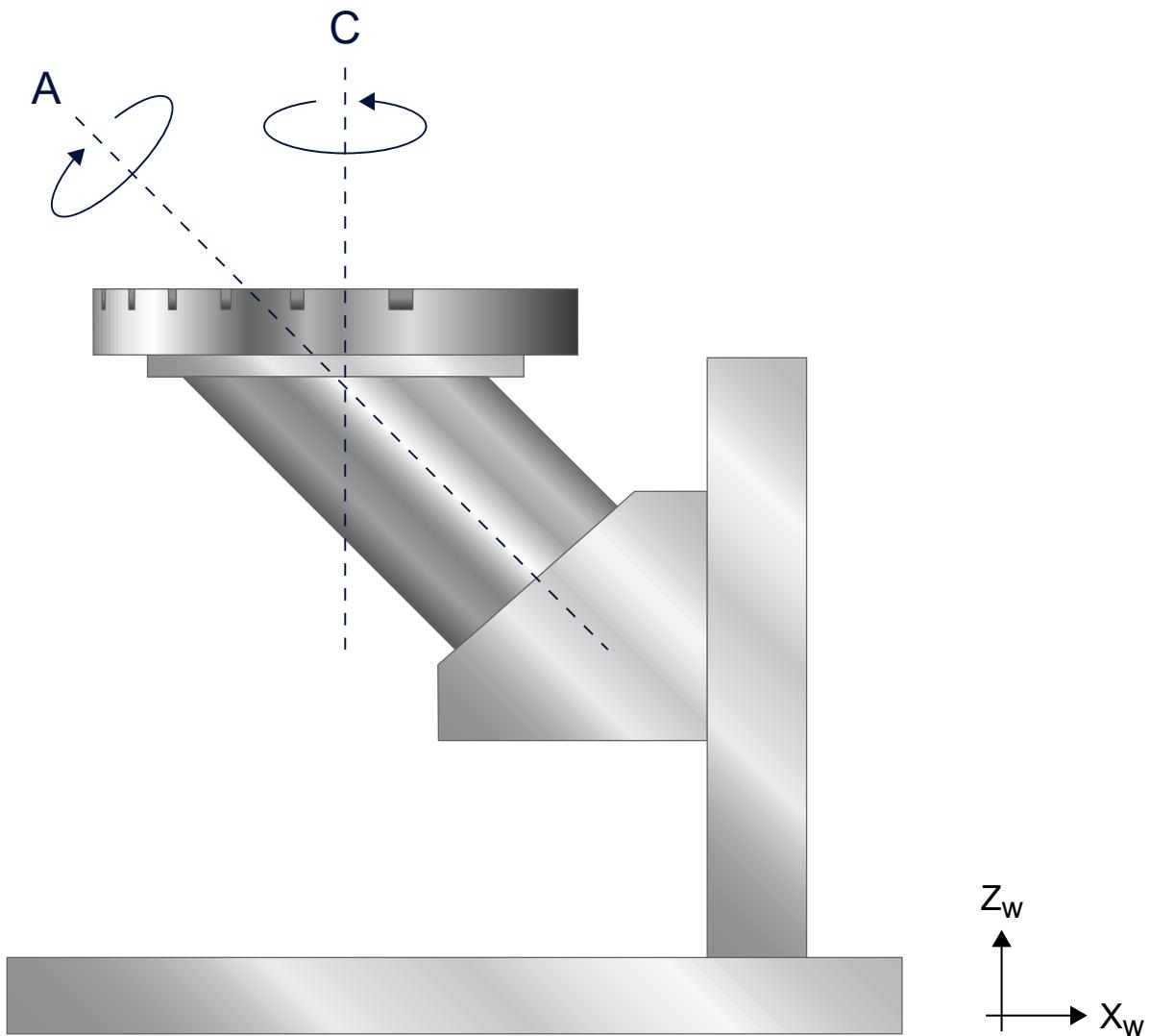
Fig. 9: Detailed view of the workpiece table
