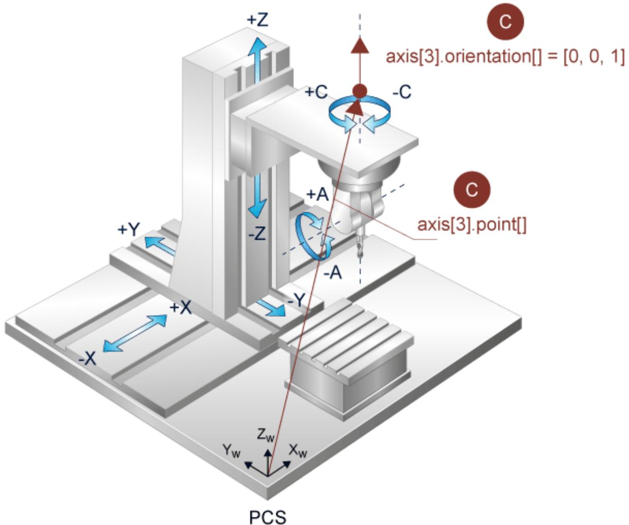
Fig. 4: Definition of the C axis
