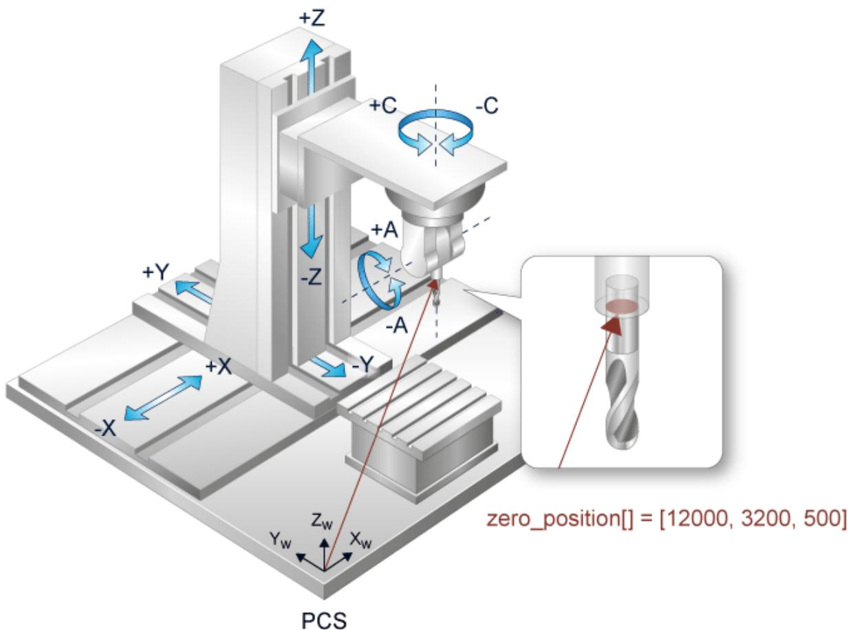
Fig. 1: Zero position of the flange
