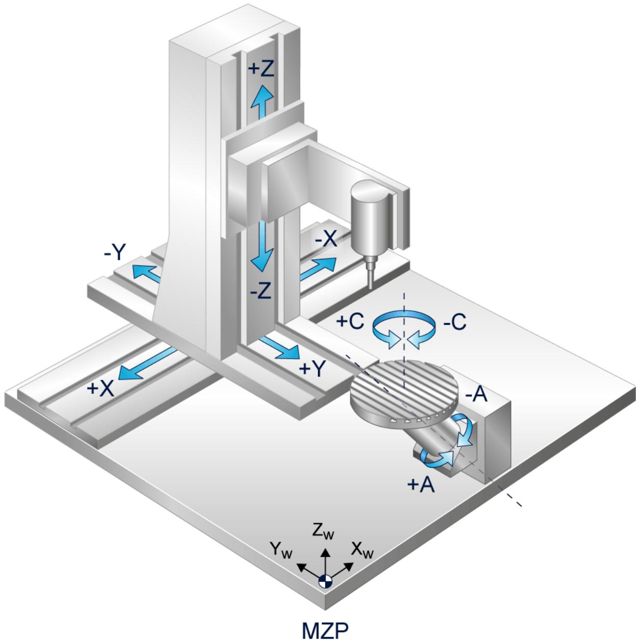
Fig. 8: Kinematics of 5-axis machine with AC workpiece table
