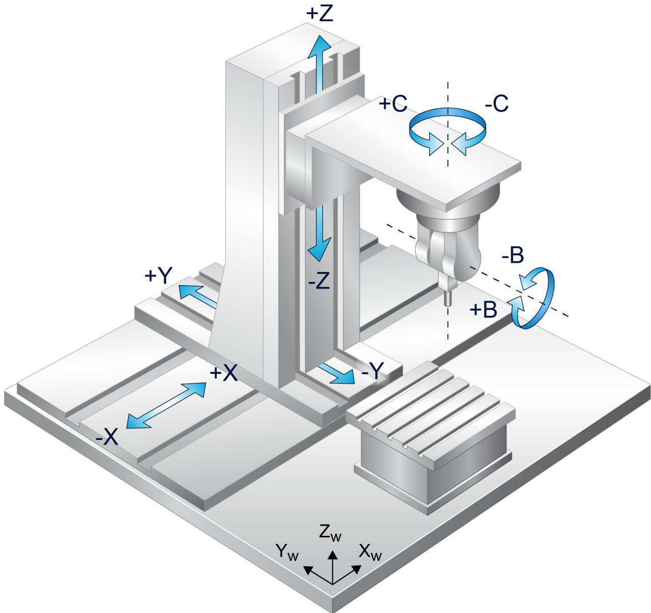
Fig. 10: CB head kinematic
