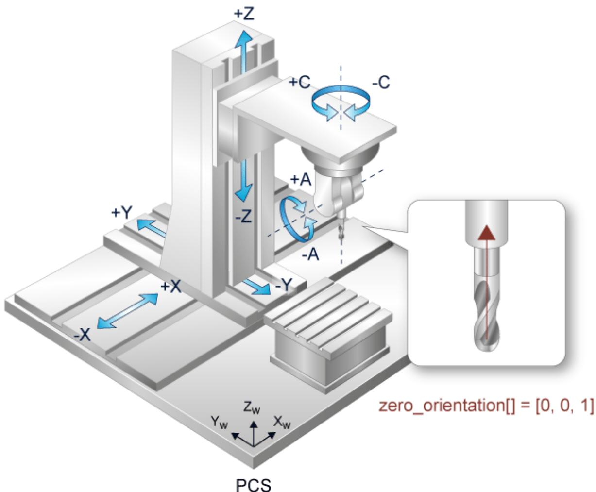
Fig. 2: Zero orientation of the tool
