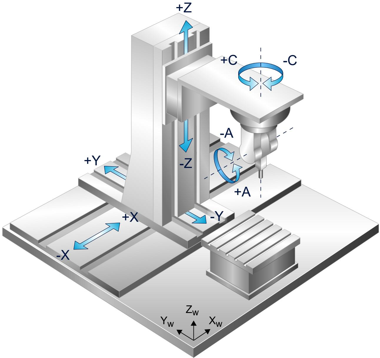
Fig. 6: Axis sequence with a CA machine
