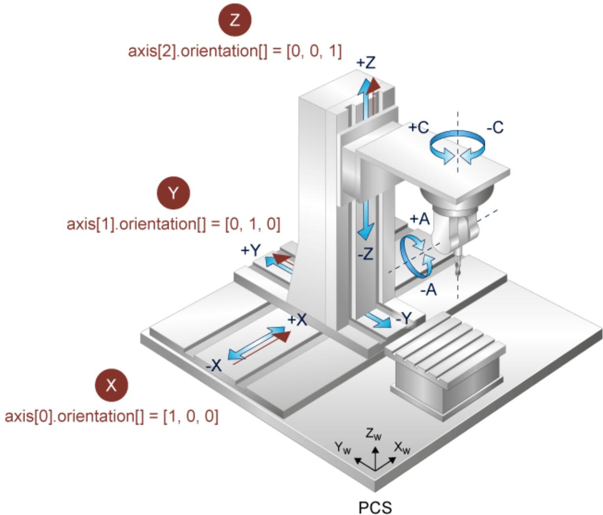
Fig. 3: Orientation of main axes
