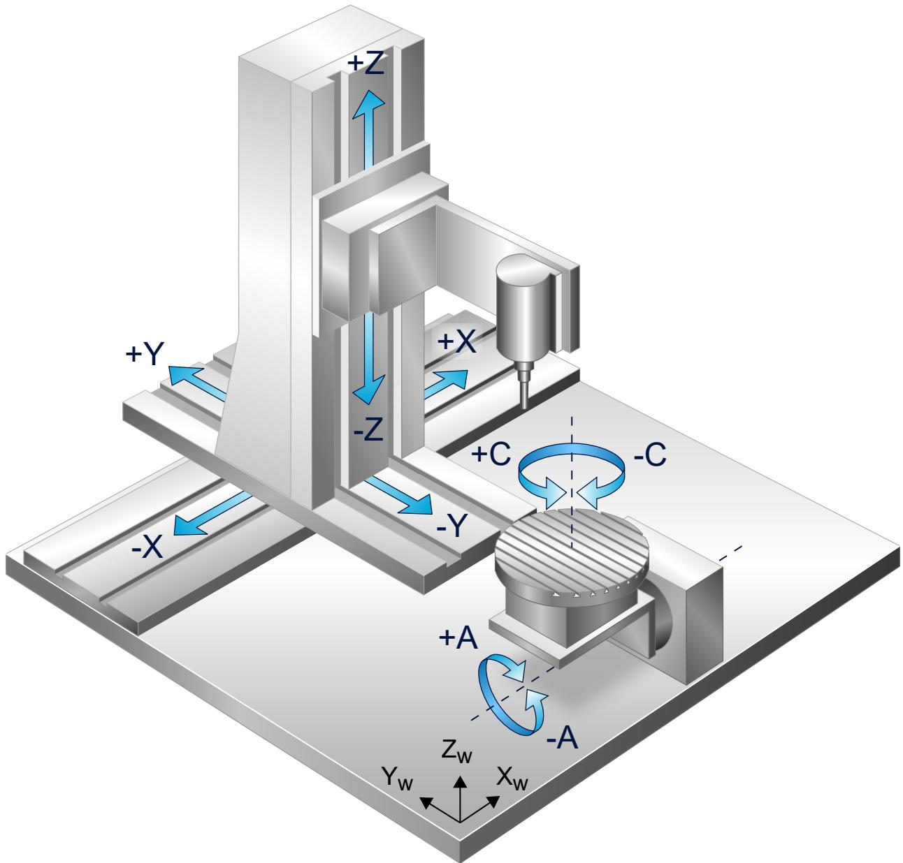
Fig. 7: Kinematics of 5-axis machine with AC workpiece table
