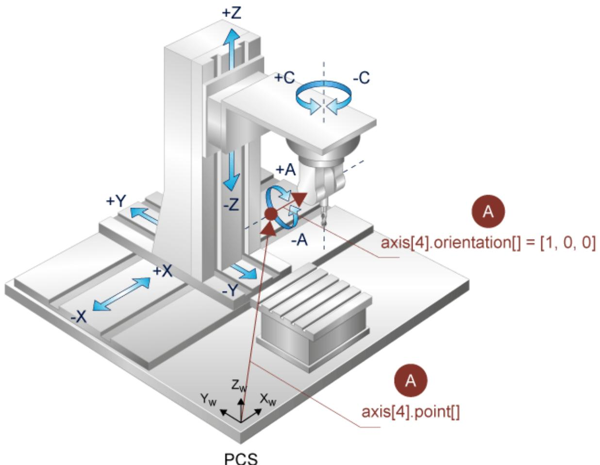
Fig. 5: Definition of A axis
