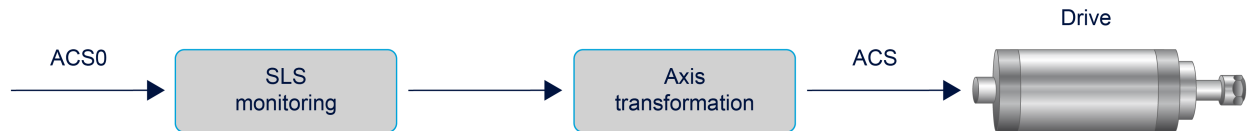
Fig. 53: Input of backward transformation with SLS monitoring
