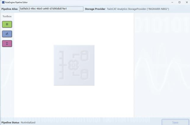
An alias can be assigned for a RuleEngine pipeline. The alias is freely selectable and can be edited via the text field at the top left of the RuleEngine Pipeline Editor.
