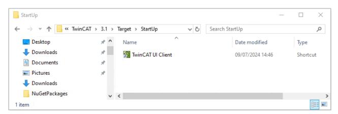
If TwinCAT is operated in configuration mode, you can create a link from the TwinCAT UI Client in your user's startup directory. You can access the folder directly using the following command (shortcut Windows + R):
