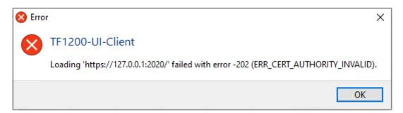
**Background**: The certificate used for the HTTPS connection is classified as insecure by Chromium because it is not known to the operating system (e.g. self-signed certificates).
