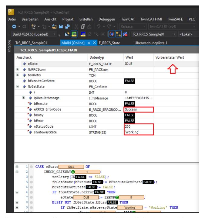
If the request was successful, the state of the eState changes back to IDLE after a few cycles and the variable sGatewayState receives the value 'Working'.
