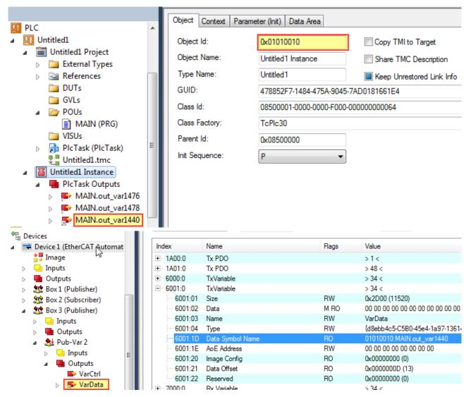
As the previous illustration shows, the symbol name is made up of the *Object ID (OID)* of the PLC instance and the unique name of the PLC program variable, separated by a colon. Using the same syntax a symbol name can also be entered for an EAP object during the online configuration. The PLC variable is then linked accordingly with the *Rx/TxVariable*.
