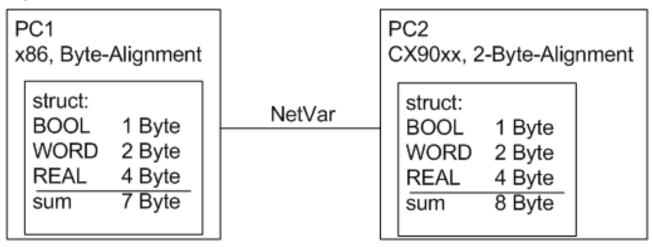
In the example (see illustration above) the structure in PC2 is larger than in PC1. Not only that, the word and real variables don't match, since a variable can begin at any byte position in PC1 but only at any evennumbered byte position in PC2.
