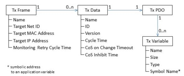
At the next higher level, TxVariables are referenced in the TxPDO elements (TxPDO = TxProcessDataObjects). A TxPDO can reference several TxVariables, thereby consolidating them in an object. The TxPDO then defines an ordered set of TxVariables. The condition that the maximum size of an EAP frame must not be exceeded also applies to a TxPDO.
