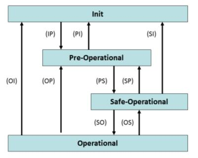
The regular state of each EAP device after it started is the **OP** state. Until the **OP** state is reached, the EAP device is switched once to each state in turn. During each state transition the EAP device performs certain actions. If an error occurs during one of the transitions, the device cannot be switched to the corresponding subsequent state and therefore remains in the state that was reached last. A readable error code can be used to diagnose the reason for the error.
