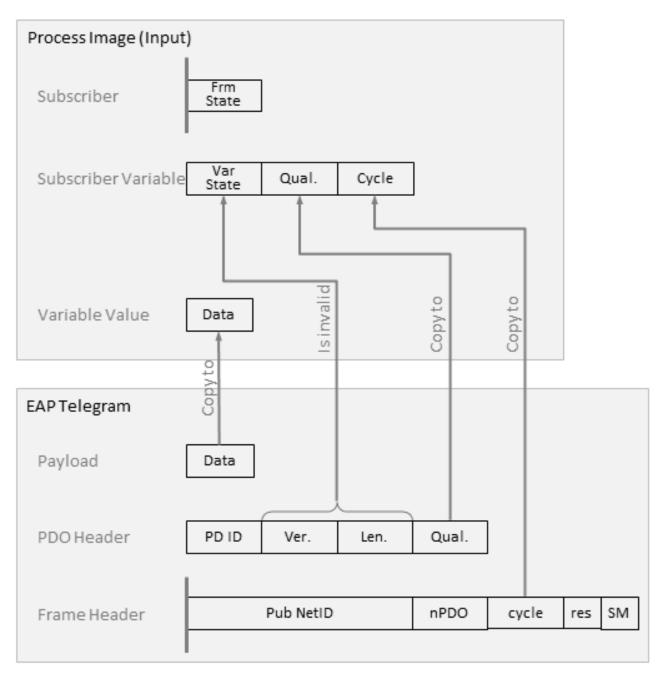
As shown in the illustration above, the received *Quality* value from the telegram, for example, is allocated to the corresponding *Quality* variable of the input process image.
