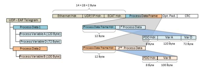
(This calculation includes 28 bytes for the UDP/IP Hdr. The 28 bytes are available for data in pure Ethernet communication.)
