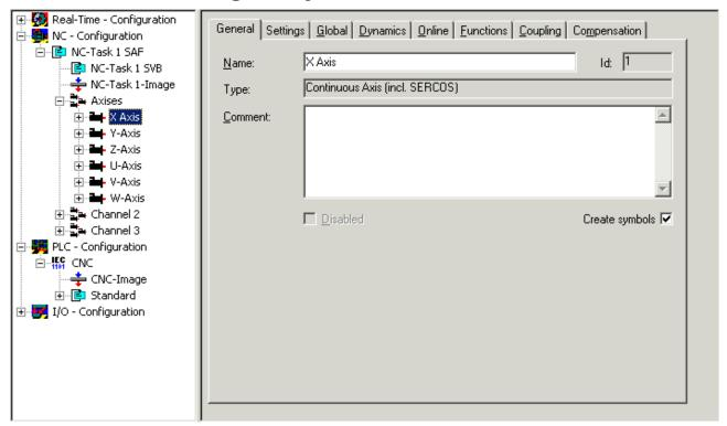
It is necessary for these to be created in order to be able to access the NC variables symbolically. This is done by activating the "Create symbols" checkbox in the System Manager. It is possible here to generate symbols for every axis. It is also possible to generate symbols for the encoder, the drive and the controller. These are not, however, generally of great importance, and should only be generated when needed.
