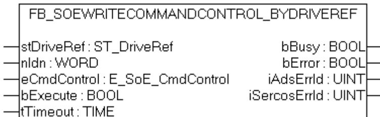
The functionblock FB\_SoEWriteCommandControl\_ByDriveRef can be used to prepare, start or cancel a command.
