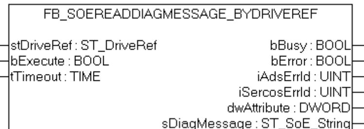
The functionblock FB\_SoEReadDiagMessage\_ByDriveRef can be used to read the diagnose message as a Sercos-String (S-0-0095).
