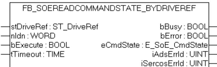
The function block FB\_SoEReadCommandState\_ByDriveRef can be used to read the state of a command.
