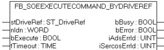
The functionblock FB\_SoEExecuteCommand\_ByDriveRef can be used to execute a command.
