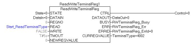
In Example 1 the terminal identifier is read from register 8 of an analog output terminal. The variables *State*, *Control*, *DataIn* and *DataOut* are linked to the terminal's corresponding I/O variables in the TwinCAT System Manager. The terminal identifier is KL**4002**..
