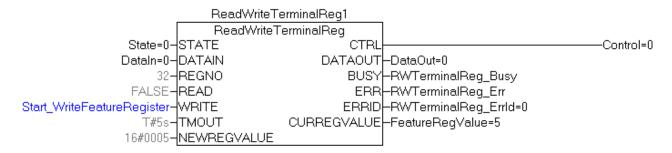
In Example 2 the user-scaling is activated in the feature register (register 32) of a KL4002 analog output terminal. The new value in the feature register is then read by the function block, and can be checked through the output variable **CURREGVALUE**.
