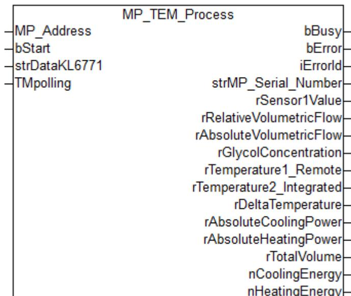
This function block is suitable for the Thermal Energy Meter type 22PE-.. and 22PEM-.... For more information please visit [www.belimo.ch](http://www.belimo.ch).
