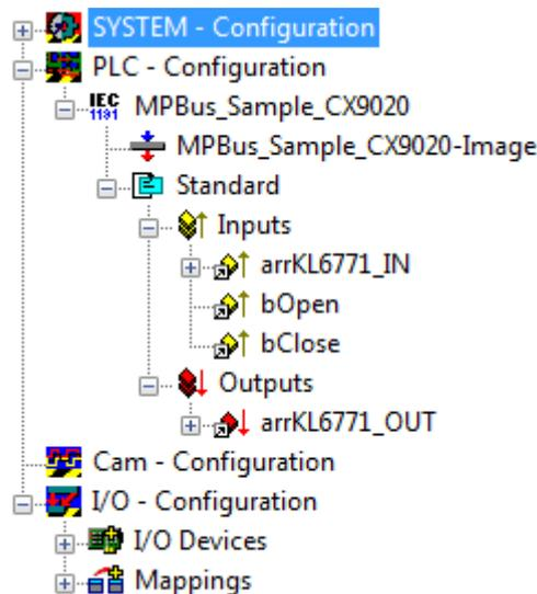
Now link the global variables of the PLC program with the Bus Terminal inputs and outputs, create the allocations, and activate the configuration. Then start the device in run mode.
