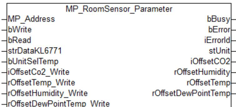
This function block is used to parameterize room sensors of types 22Rxx-19-1 that were produced before May 2022 (as of May 2022, see [MP\\_OperatingUnit\\_Configuration](#)).
