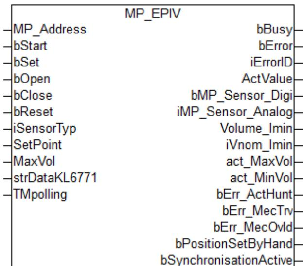
This function block is used to control a pressure-independent control ball valve. For more information please visit [www.belimo.ch](http://www.belimo.ch).
