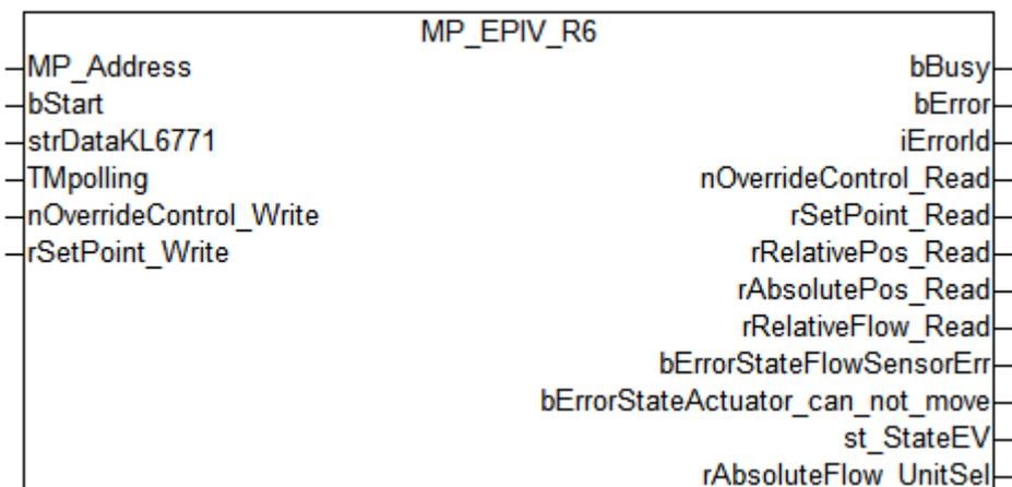
This function block is used to control a control ball valve of series EP..R-R6+BAC.
