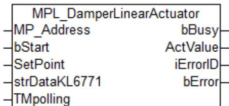
This function block is used to control and monitor an actuator of a damper and of a globe valve.
