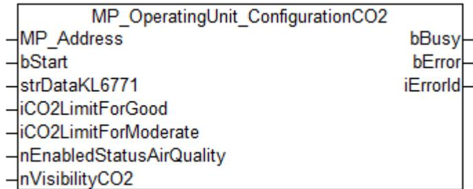
This function block is used to configure room sensors of types P-22Rxx-1900x-1. It is compatible with 22Rxx-19-1 room sensors produced as of May 2022 (before May 2022, see [MP RoomSensor Parameter](#) [► 55]).
