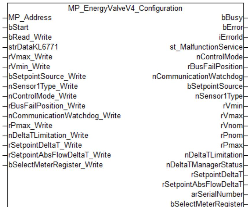
This function block is used to configure the Energy Valve actuators EV..R2+... (V4). For more information please visit [www.belimo.ch](http://www.belimo.ch).
