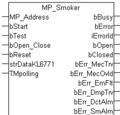
This function block is used to control and monitor a fire damper.
