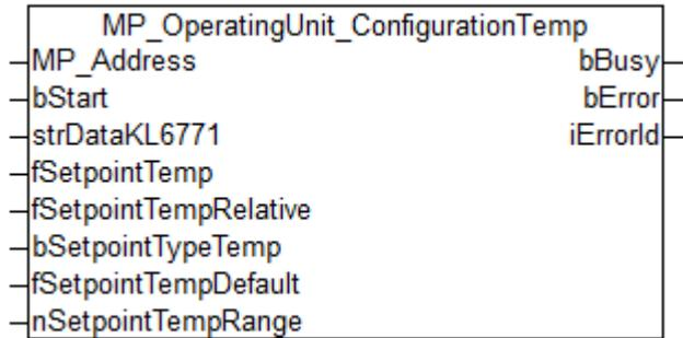
This function block is used to configure room sensors of types P-22Rxx-1900x-1. It is compatible with 22Rxx-19-1 room sensors produced as of May 2022 (before May 2022, see [MP\\_RoomSensor\\_Parameter \[▶ 55\]](#)).
