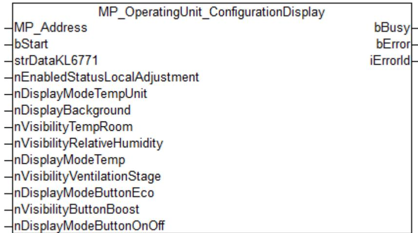
This function block is used to configure room sensors of types P-22Rxx-1900x-1. It is compatible with 22Rxx-19-1 room sensors produced as of May 2022 (before May 2022, see [MP\\_RoomSensor\\_Parameter](#) [► 55]).
