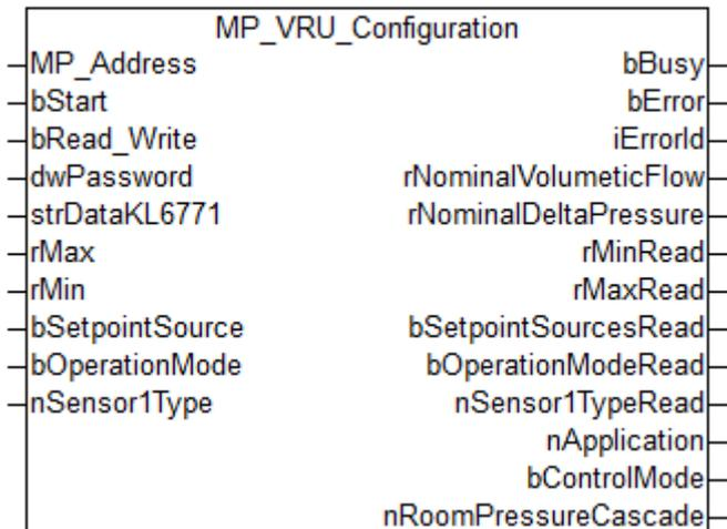
This function block is used to configure the VAV actuators VRU-D3-BAC, VRU-M1-BAC and VRU-M1R-BAC (max. 8 slaves). Further information can be found at [www.belimo.ch](http://www.belimo.ch).
