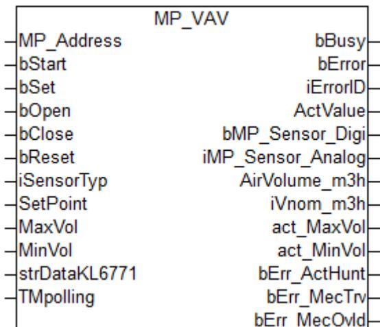
This function block is used to control and monitor a volume flow controller.
