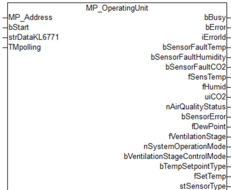
This function block is used to read room sensors of types P-22Rxx-1900x-1. It is compatible with 22Rxx-19-1 room sensors produced as of May 2022 (before May 2022, see [MP\\_RoomSensor \[▶ 54\]](#)).
