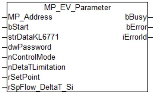
This function block is used for parameterization of valves.
