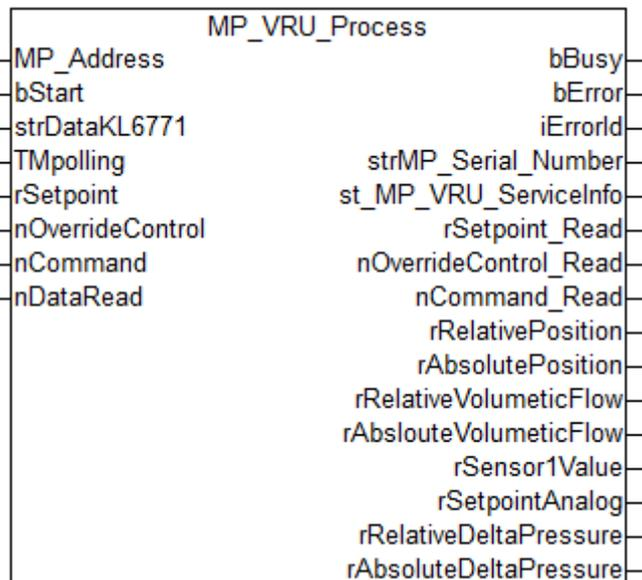
This function block is suitable for VAV actuators VRU-D3-BAC, VRU-M1-BAC and VRU-M1R-BAC (max. 8 slaves). For more information please visit [www.belimo.ch](http://www.belimo.ch).
