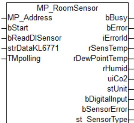
This function block is used to read out room sensors of types 22Rxx-19-1 that were produced before May 2022 (as of May 2022, see MP\_OperatingUnit [▶ 45]).
