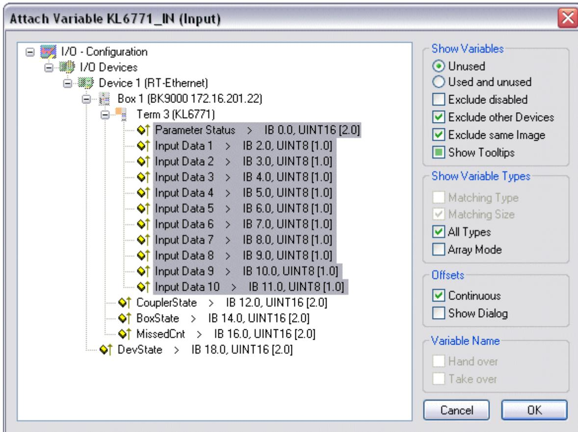
4. You can now check the link. To do this, go to the KL6771 and open it. All the terminal's data should now be marked by a small arrow (see Figure).
