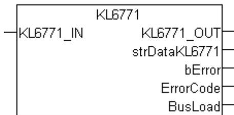
This function block takes care of communication with the KL6771 MP-Bus master terminal. The KL6771 is configured with this function block, and data exchange with the MP network is started.
