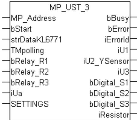
This function block is used to control and monitor a multi-I/O module UST3.
