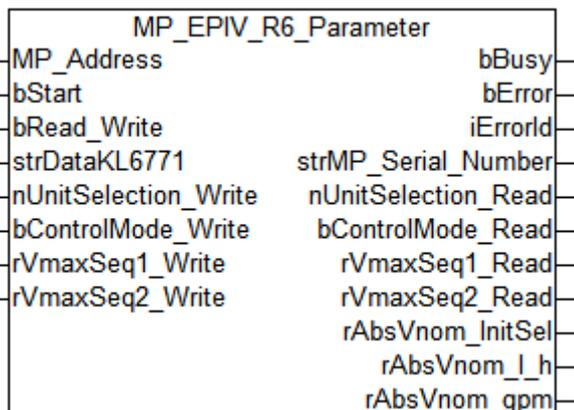
This function block is used for parameterization of valves of EP..R-R6+BAC series.
