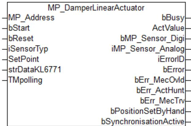
This function block is used to control and monitor an actuator of a damper and of a globe valve.
