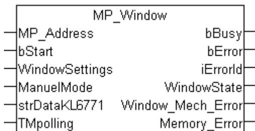
This function block is used to control and monitor a window ventilation system (FLS).
