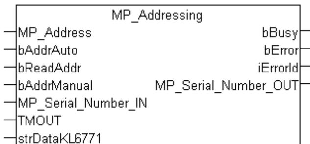
This function block allows an MP-Bus slave to be addressed. It is also possible to use this function block to read the serial number of the slave.
