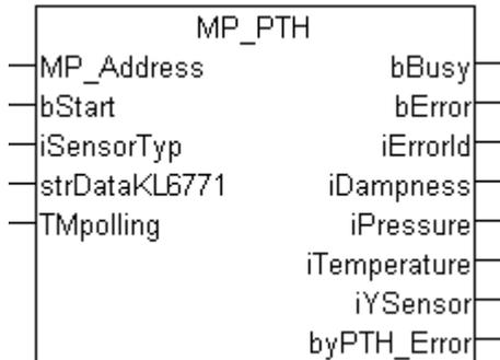
This function block is used to control and monitor a PTH sensor.
