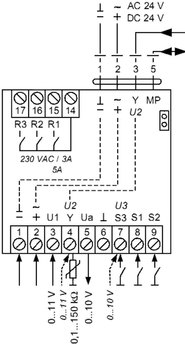
The input data **bRelay\_R1** to **bRelay\_R3** switch the relays R1 to R3 (PIN 15 to PIN 17). The variable **iUa** switches the analog output 0...10 V to PIN 5. One digit corresponds to 1 mV.
