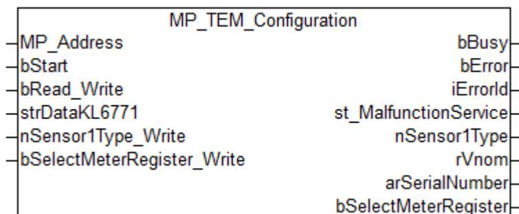
This function block is used to configure the Thermal Energy Meter type 22PE-.. and 22PEM-... . For more information please visit [www.belimo.ch](http://www.belimo.ch).
