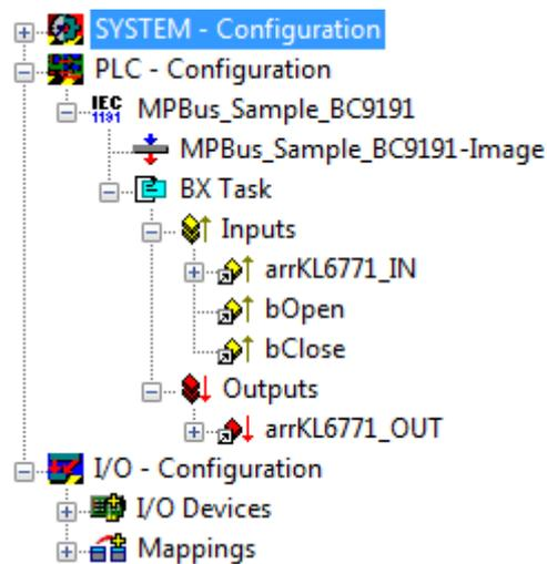
Now link the global variables of the PLC program with the Bus Terminal inputs and outputs, create the allocations, and activate the configuration. Then start the device in run mode.
