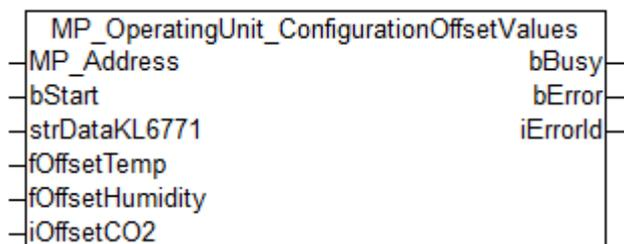
This function block is used to configure room sensors of types P-22Rxx-1900x-1. It is compatible with 22Rxx-19-1 room sensors produced as of May 2022 (before May 2022, see [MP\\_RoomSensor\\_Parameter](#) [▶ 55]).
