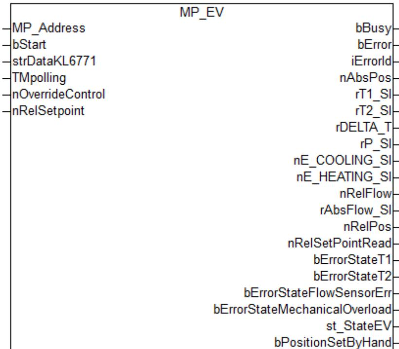
This function block is used to control a control ball valve of series P6...W..EV-BAC. For more information please visit [www.belimo.ch](http://www.belimo.ch).
