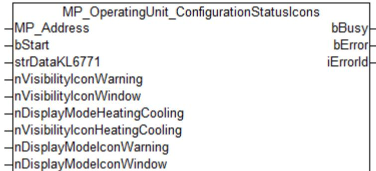
This function block is used to configure room sensors of types P-22Rxx-1900x-1. It is compatible with 22Rxx-19-1 room sensors produced as of May 2022 (before May 2022, see [MP\\_RoomSensor\\_Parameter](#) [► 55]).
