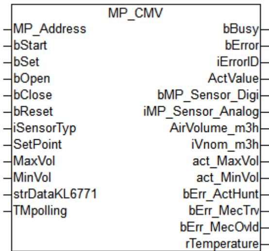
This function block is used to control and monitor a volume flow controller.
