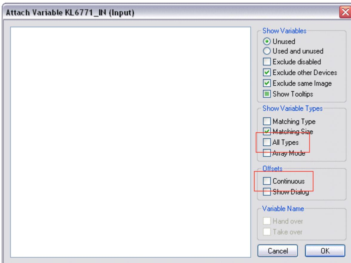
2. Click the mouse on the first variable in the KL6771 **Parameter Status**. Then press the [SHIFT] key, and hold it down. Take the mouse pointer to the last variable in the KL6771 **Input Data 10**, and again click the left mouse button. Now release the [SHIFT] key again.
