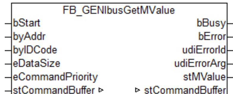
This function block reads a measured value from a GENIbus device. The operation is thereby exclusively restricted to values of class 2. Only the ID code of the high byte and the length of the measured value need to be specified; the type of scaling and the unit of the measured value are determined by an internal INFO query. A structure at the *stMValue* output provides all important information about the value.
