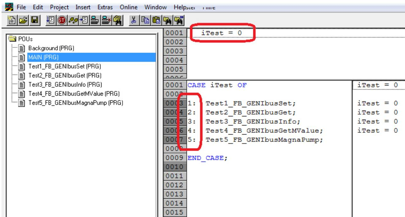
In the respective program sections, function blocks are then prepared that you can operate via the test inputs *ib1* to *ib8*:
