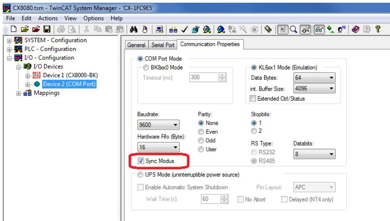
The activation of the “Sync Mode” is particularly important. This ensures that the interface, which only emulates, also works correctly under higher PLC loads.
