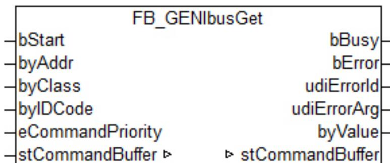
This function block reads a value from a GENIbus device.
