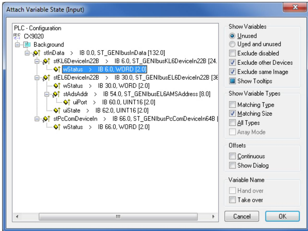
After that the data bytes can be conveniently linked to the corresponding variables by multi-link. The selection of several variables can be achieved by clicking on "Data1" and pressing the ↓ key with the Shift key pressed.
