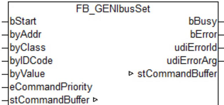
This function block writes a value in a GENIbus device or executes a command (Class-3 IDs).
