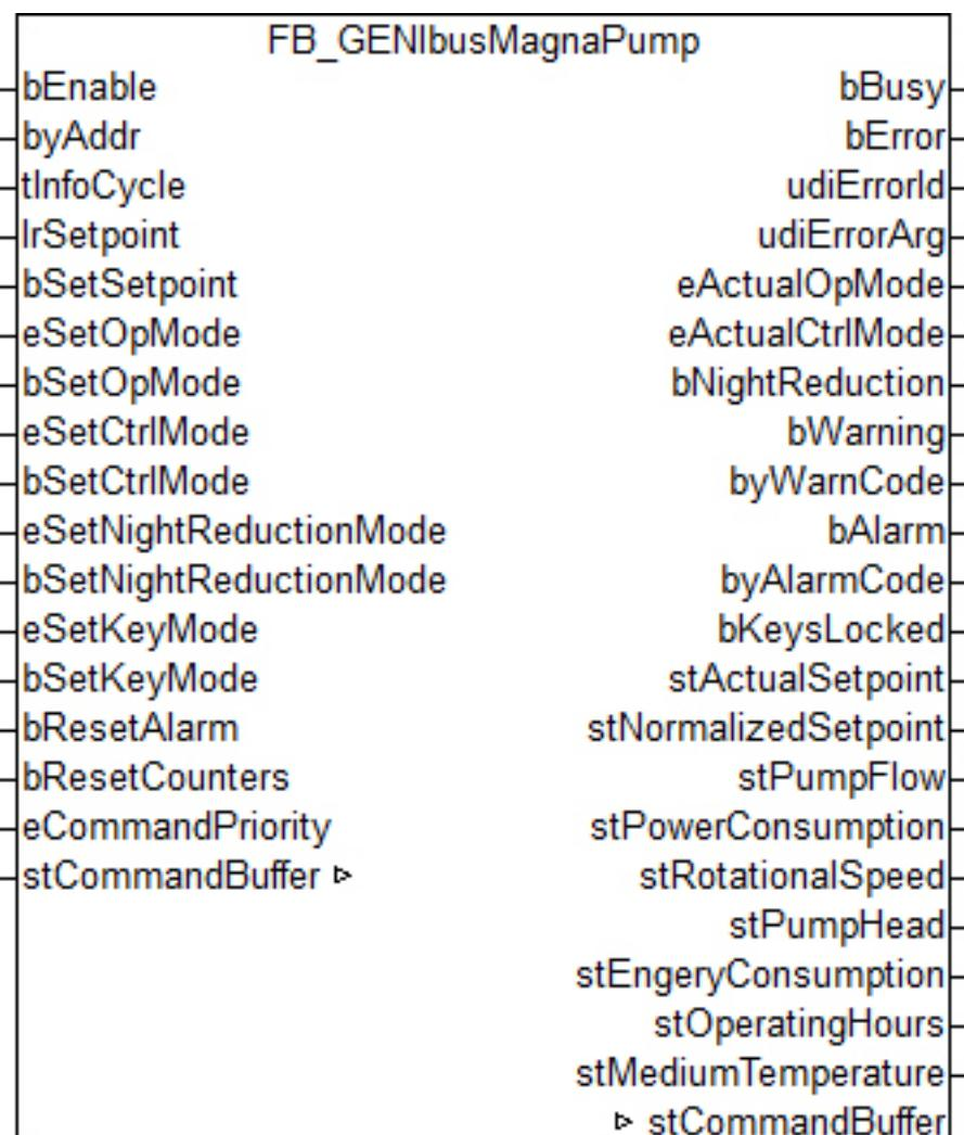
This function block represents a universal application for a Grundfos Magna pump. The fundamental operating modes can be set and important parameters read out.
