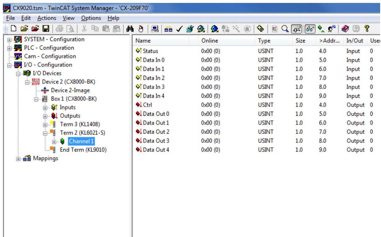
First, just the status is linked with the status variable of the communication input. Note that when doing so the structure for PC communication must be selected.
