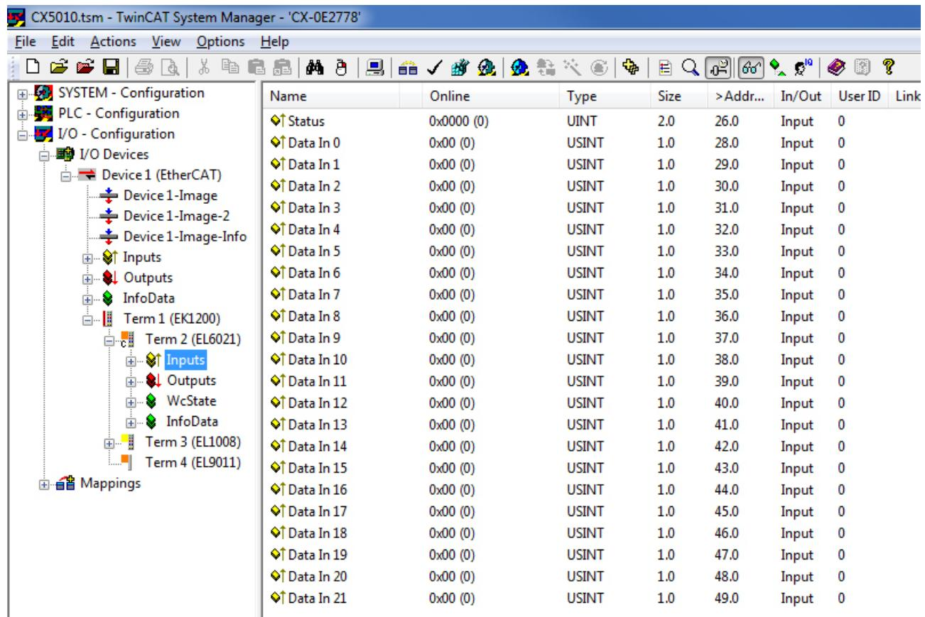
First, just the status is linked with the status variable of the communication input. Note that when doing so the structure for PC communication must be selected.
