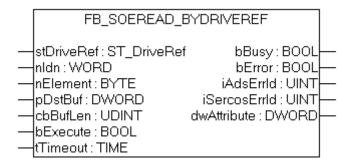
The function block FB\_SoeRead\_ByRef allows to read drive parameters with the "Servo Drive Profile over EtherCAT"(SoE) protocol. This requires the slave to have a mailbox and to support the SoE protocol. The parameter to be read is specified by the parameters nldn (Identification number), nElement and stDriveRef.
