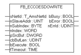
The FB\_EcCoeSdoWrite function block permits an object from the object directory of an EtherCAT slave to be written by means of an SDO download. This requires the slave to have a mailbox and to support the "CANopen over EtherCAT" (CoE) protocol. The nSubIndex and nIndex parameters select the object the data should be written to.
